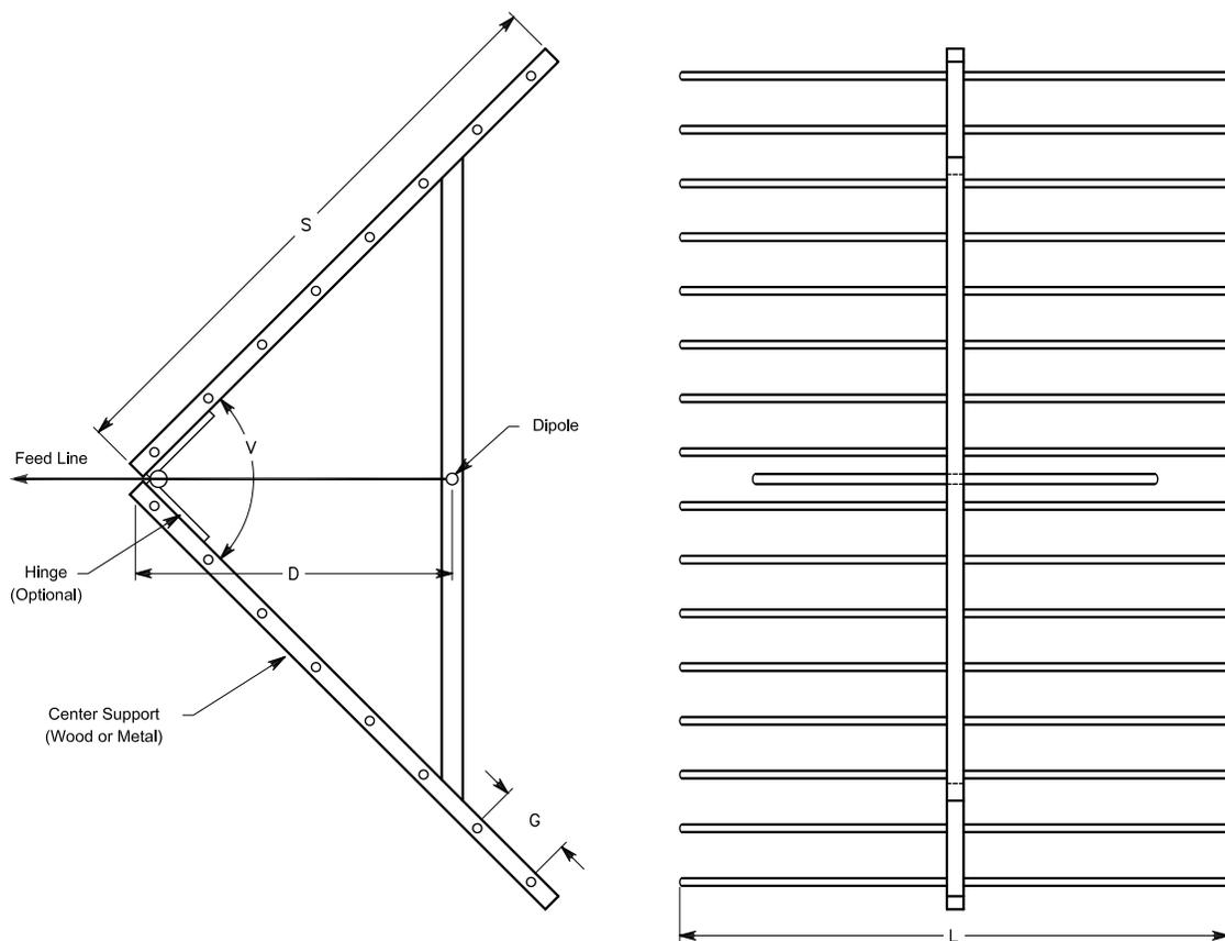
**Fig 19—Construction of a corner reflector array. The frame can be wood or metal. Reflector elements are stiff wire or tubing. Dimensions for several bands are given in Table 2. Reflector element spacing, G, is the maximum that should be used for the frequency; closer spacings are optional. The hinge permits folding for portable use.**
