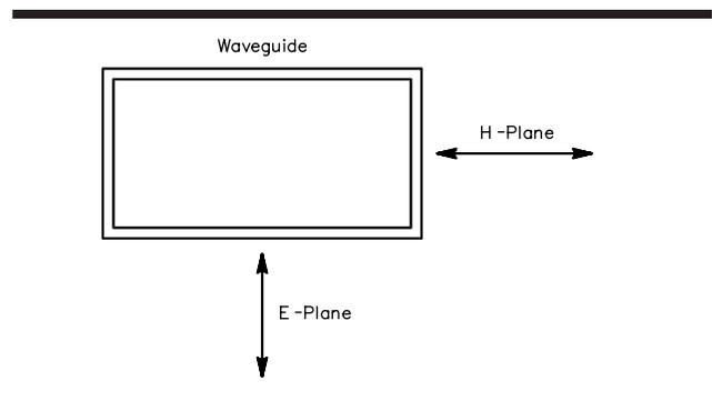
**Fig 74**—10-GHz antennas are usually fed with waveguide. See text for a discussion of waveguide propagation characteristics.
