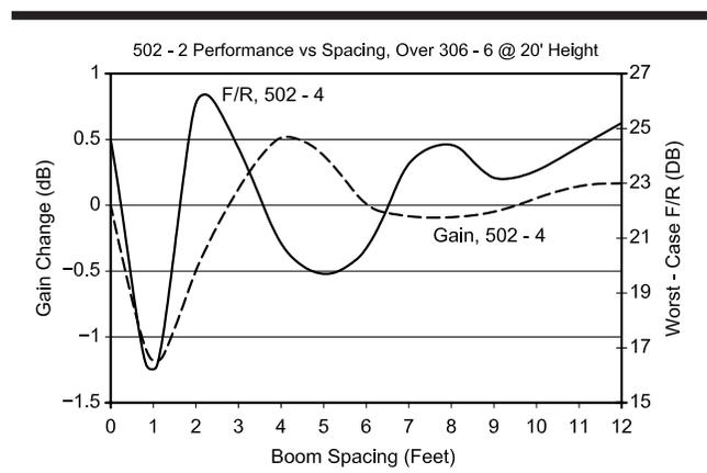
**Fig 12—** Plot of gain and worst-case F/R of a 5-element 2-meter Yagi on a 4-foot boom as a function of distance over a 3-element 6-meter beam on a 6-foot boom. Beyond a spacing of about 3 feet the performance is degraded a minimal amount.
