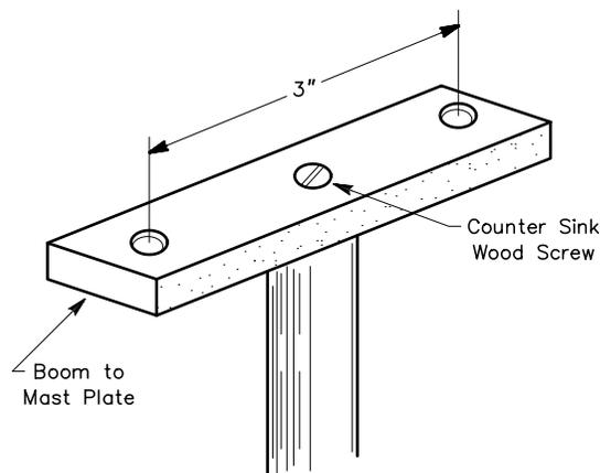
**Fig 62**—Boom to mast plate for the 144-MHz quad. The screw hole in the center of the plate should be countersunk so the wood screw attaching it to the mast does not interfere with the fit of the boom.
