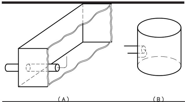
**Fig 2—Coupling coaxial line to waveguide and resonators.**
