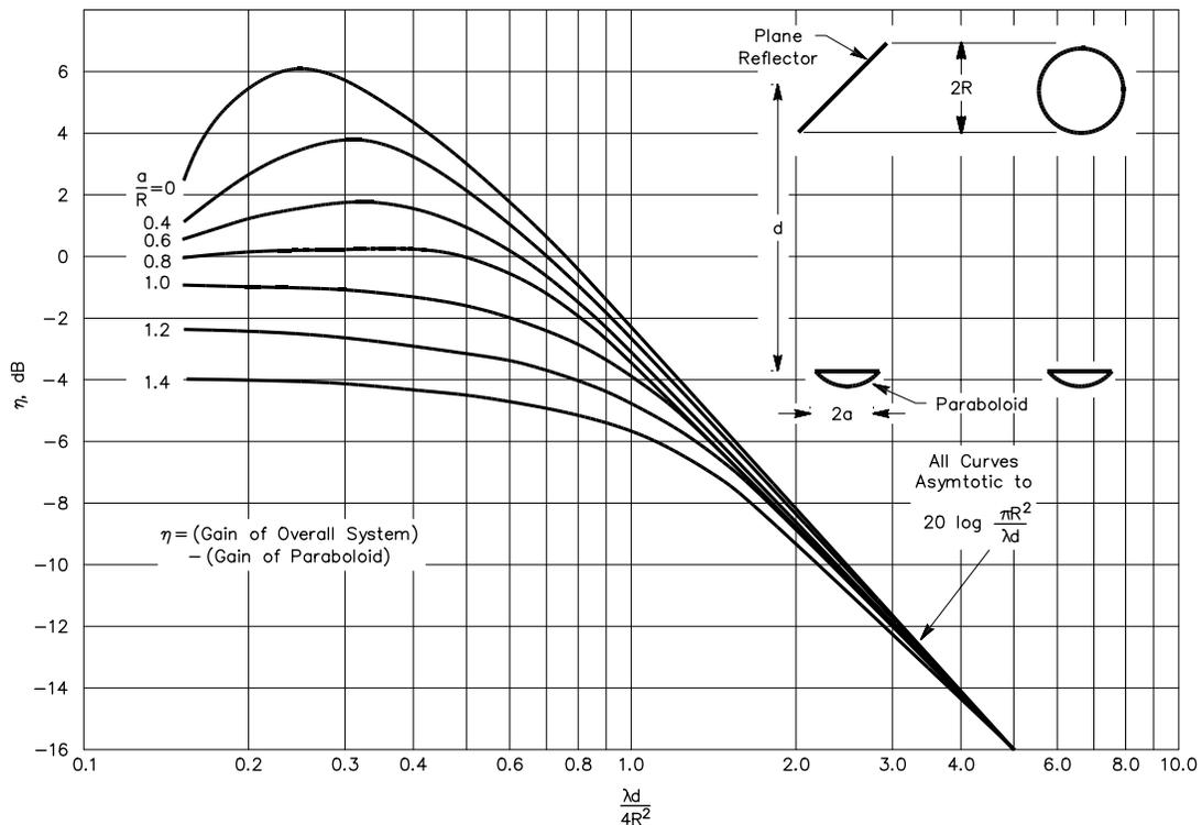
Fig 80—Gain of a periscope antenna using a plane elliptical reflector (after Jasik—see Bibliography).
