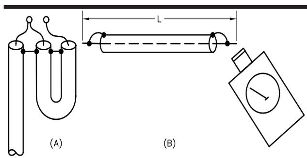
**Fig 5—Conversion from unbalanced coax to a balanced load can be done with a  $\frac{1}{2}\lambda$ , coaxial balun at A. Electrical length of the looped section should be checked with a dip meter, with the ends shorted, as at B. The  $\frac{1}{2}\lambda$  balun gives a 4:1 impedance step-up.**
