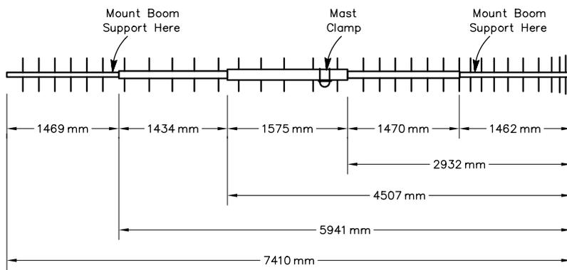
**Fig 46—Boom-construction information for the 33-element Yagi. Lengths are given in millimeters to allow precise duplication of the antenna.**
