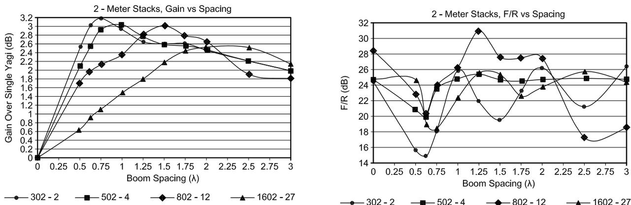
**Fig 15—Performance of two different 2-meter Yagis (5-elements on 4-foot boom and 8-elements on 12-foot boom) fed in-phase, as a function of spacing between the booms. Note that the distance is measured in wavelengths.**
