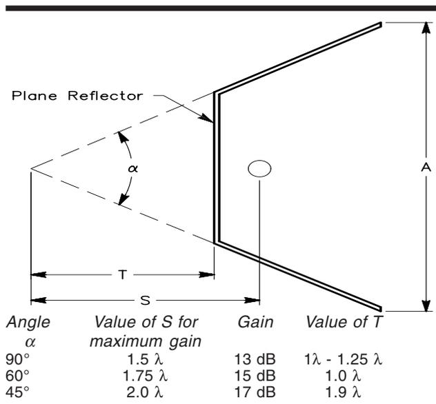
**Fig 21—The trough reflector.** This is a useful modification of the corner reflector. The vertex has been cut off and replaced by a simple plane section. The tabulated data shows the gain obtainable for greater values of S than those covered in Table 2, assuming that the reflector is of adequate size.
