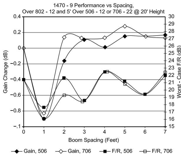
**Fig 13**—Performance of a 14-element 70-cm Yagi on a 9-foot boom, mounted a variable distance over an 8-element 2-meter Yagi on a 12-foot boom, which is mounted 5 feet above either a 5-element 6-meter Yagi on a 12-foot boom or a 7-element 6-meter Yagi on a 22-foot boom. Beyond a spacing of about 4 feet, the performance of the 70-cm beam is degraded a minimal amount.
