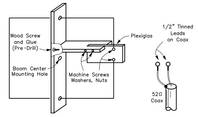
Fig 60—Layout of the driven element of the 144-MHz quad. The leads of the coaxial cable should be stripped to  $\frac{1}{2}$  in. and solder lugs attached for easy connection and disconnection. See text regarding impedance at loop support points.
