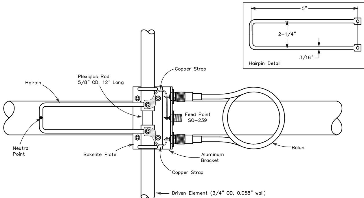
**Fig 36**—This shows how the driven element and feed system are attached to the boom. The phasing line is coiled and taped to the boom. The center of the hairpin loop may be connected to the boom electrically and mechanically if desired.
