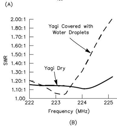
**Fig 54—H- and E-plane patterns for the 16-element 222-MHz Yagi at A. The driven-element T-match dimensions were chosen for the best SWR compromise between wet and dry weather conditions. The SWR vs frequency curve shown at B demonstrates the broad frequency response of the Yagi design.**
