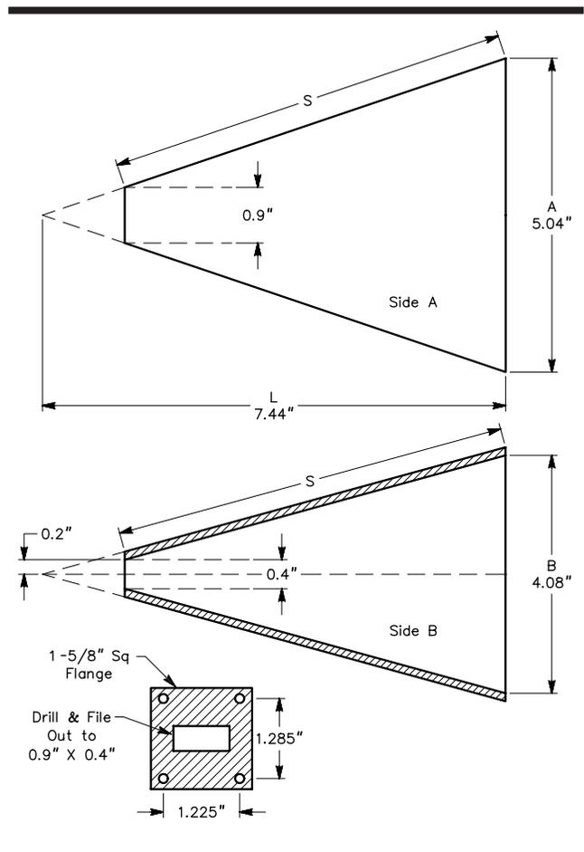
**Fig 77**—Dimensions of the brass pieces used to make the 10-GHz horn antenna. Construction requires two of each of the triangular pieces (side A and side B).
