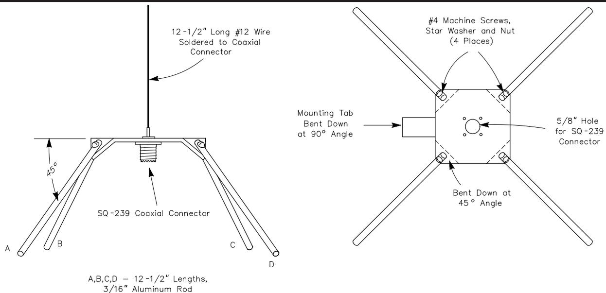
**Fig 31**—Dimensional information for the 222-MHz ground-plane antenna. Lengths for A, B, C and D are the total distances measured from the center of the SO-239 connector. The corners of the aluminum plate are bent down at a 45° angle rather than bending the aluminum rod as in the 144-MHz model. Either method is suitable for these antennas.
