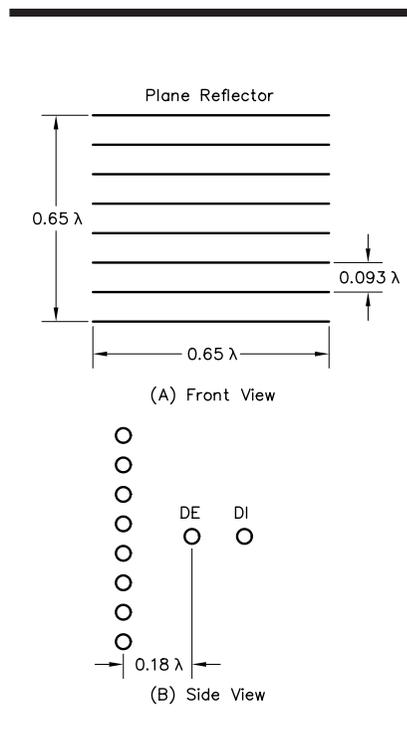
**Fig 38**—Front and side views of a plane-reflector antenna.
