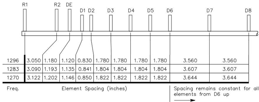
**Fig 69—Boom drilling dimensions.** These dimensions must be carefully followed and the same materials used if performance is to be optimum. Element spacings are the same for all directors after D6—use as many as necessary to fill the boom.
