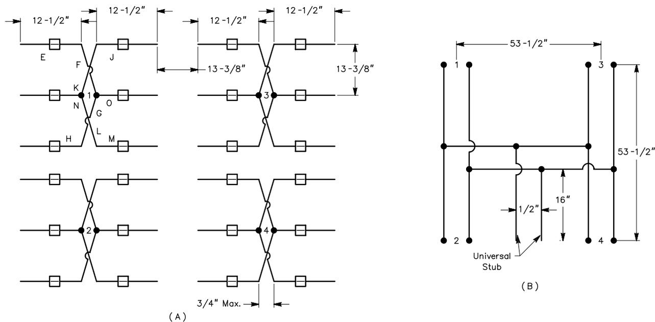
**Fig 17**—Large collinear arrays should be fed as sets of no more than eight driven elements each, interconnected by phasing lines. This 48-element array for 432 MHz (A) is treated as if it were four 12-element collinear antennas. Reflector elements are omitted for clarity. The phasing harness is shown at B. Squares represent insulators.
