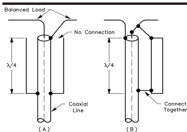
**Fig 6—The balun conversion function, with no impedance transformation, can be accomplished with  $\frac{1}{4}\lambda$  lines, open at the top and connected to the coax outer conductor at the bottom. The coaxial sleeve at A is preferred.**
