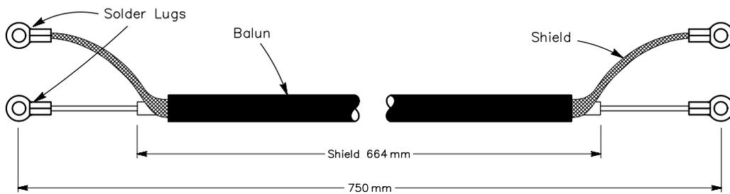
Material: RG-142/U or RG-303/U Teflon-Insulated Coaxial Cable
