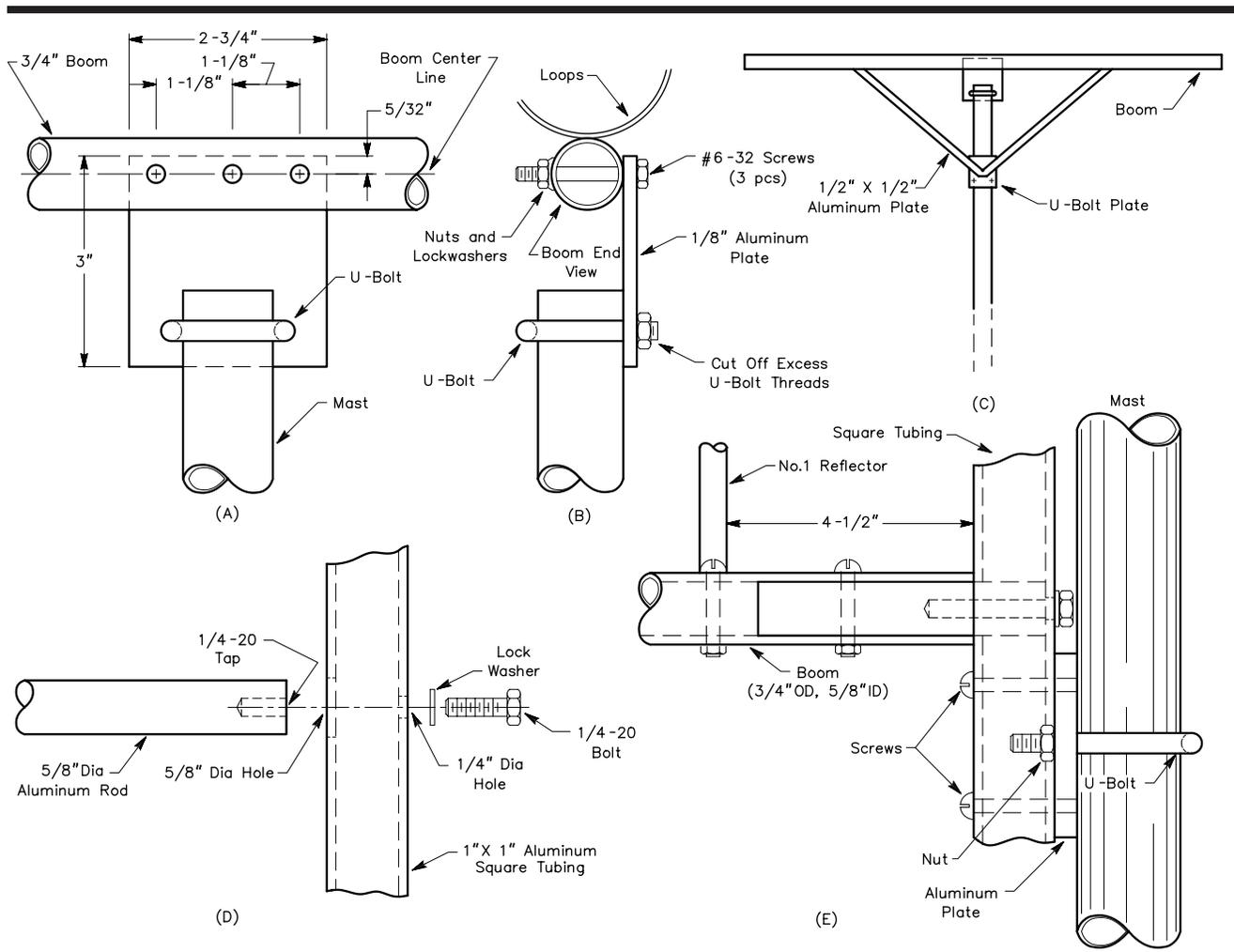
**Fig 68**—Loop Yagi boom-to-mast plate details are given at A. At B, the mounting of the antenna to the mast is detailed. A boom support for long antennas is shown at C. The arrangement shown in D and E may be used to rear-mount antennas up to 6 or 7 ft long.
