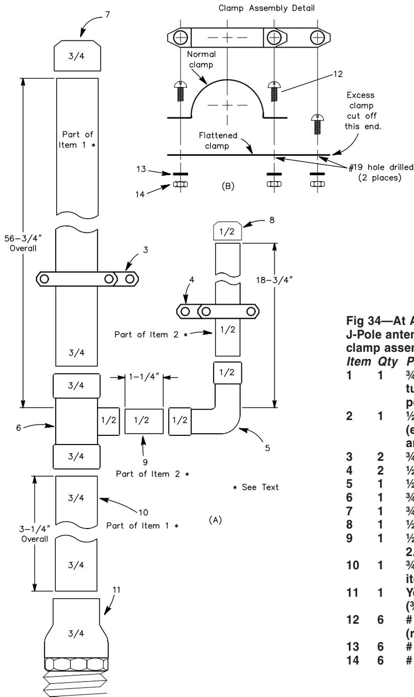
Fig 34—At A, exploded assembly diagram of all-copper J-Pole antenna. At B, detail of clamp assemblies. Both clamp assemblies are the same.
