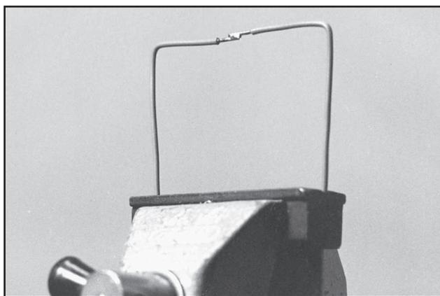
**Fig 67**—These photos show the construction method used for the 1296-MHz quad type parasitic elements. The two ends of the #18 bell wire are brought together with an overlap of  $\frac{1}{8}$  in. and soldered.
