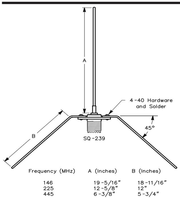
**Fig 32—Simple ground-plane antenna for the 144-, 222- and 440-MHz bands. The vertical element and radials are  $\frac{3}{32}$ - or  $\frac{1}{16}$ -in. brass welding rod. Although  $\frac{3}{32}$ -in. rod is preferred for the 144-MHz antenna, #10 or #12 copper wire can also be used.**
