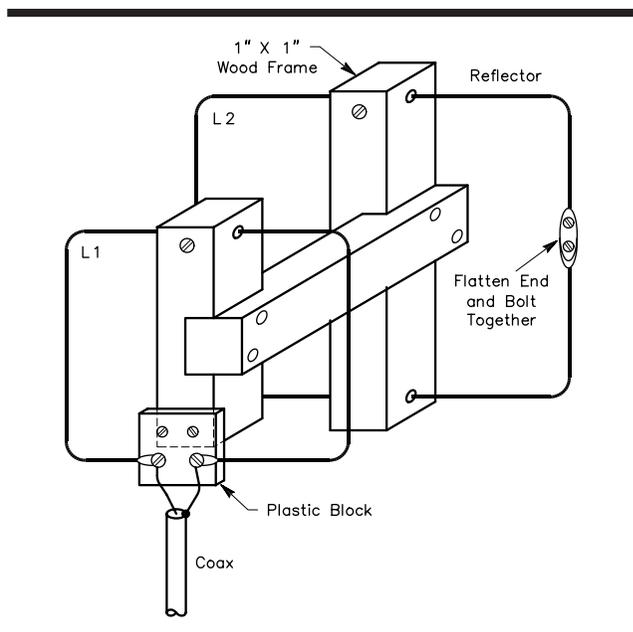
**Fig 55—Mechanical details of a 2-element quad for 144 MHz. The driven element, L1, is one wavelength long; reflector L2 is 5% longer. With the transmission line connected as shown here, the resulting radiation is horizontally polarized. Sets of elements of this type can be stacked horizontally and vertically for high gain with broad frequency response. Recommended bay spacing is  $\frac{1}{2} \lambda$  between adjacent element sides. The example shown may be fed directly with 50-Ω coax.**
