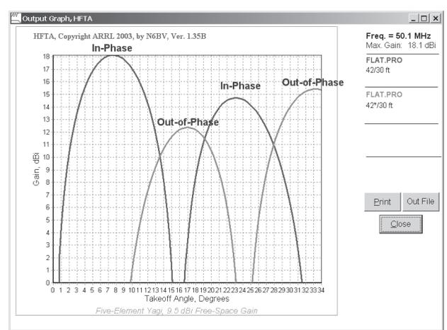
**Fig 14**—*HFTA* comparison plots of the elevation responses for two 5-element 6-meter Yagis mounted at 42 and 30 feet above flat ground, when they are fed in-phase and out-of-phase. By switching the phasing (adding a half-wavelength of coax to one of the antennas), the elevation angle can be controlled to enhance performance when a Sporadic-E cloud is nearly overhead.
