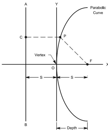
**Fig 24—Details of the parabolic curve,  $Y^2 = 4SX$ . This curve is the locus of points that are equidistant from a fixed point, the focus (F), and a fixed line (AB) that is called the *directrix*. Hence,  $FP = PC$ . The focus (F) is located at coordinates S,0.**
