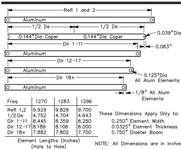
**Fig 70—Parasitic elements for the loop Yagi are made from aluminum sheet, the driven element from copper sheet.** The dimensions given are for 1/4-in. wide by 0.0325-in. thick elements only. Lengths specified are hole to hole distances; the holes are located 1/8 in. from each element end.
