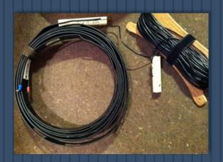
Attach the feed point of the ladder line with the long wire radiator to the positive side of the balun. Attach the other leg of the ladder line feed point to the negative side of the balun. Connect the balun to your tuner. The length of coax from the balun to the tuner is not critical.
