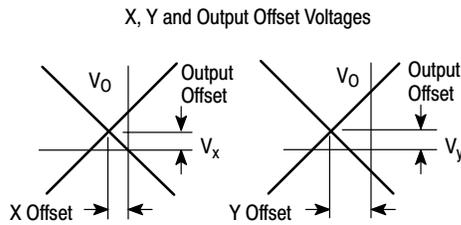
For most dc applications, all three offset adjust potentiometers ( $P_1$ ,  $P_2$ ,  $P_4$ ) will be necessary. One or more offset adjust potentiometers can be eliminated for ac applications (see Figures 28, 29, 30, 31).
