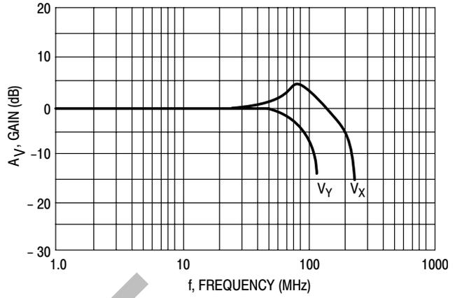
Figure 2. Transconductance Bandwidth
