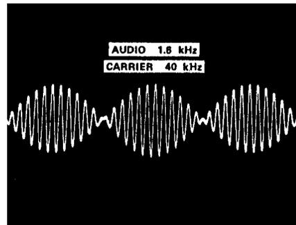
Figure 29. Balanced Modulator
