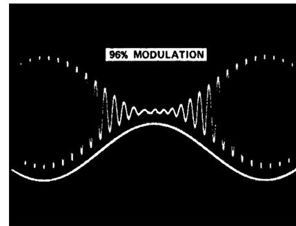
Figure 30. Amplitude Modulation
