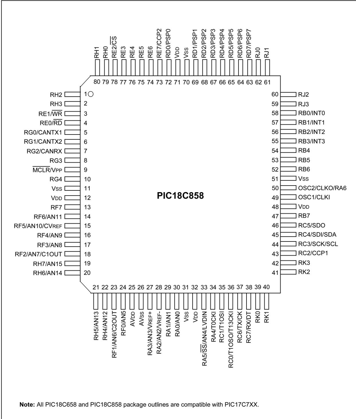
**FIGURE 1-7: PIC18C858 84-PIN PLCC DIAGRAM**
