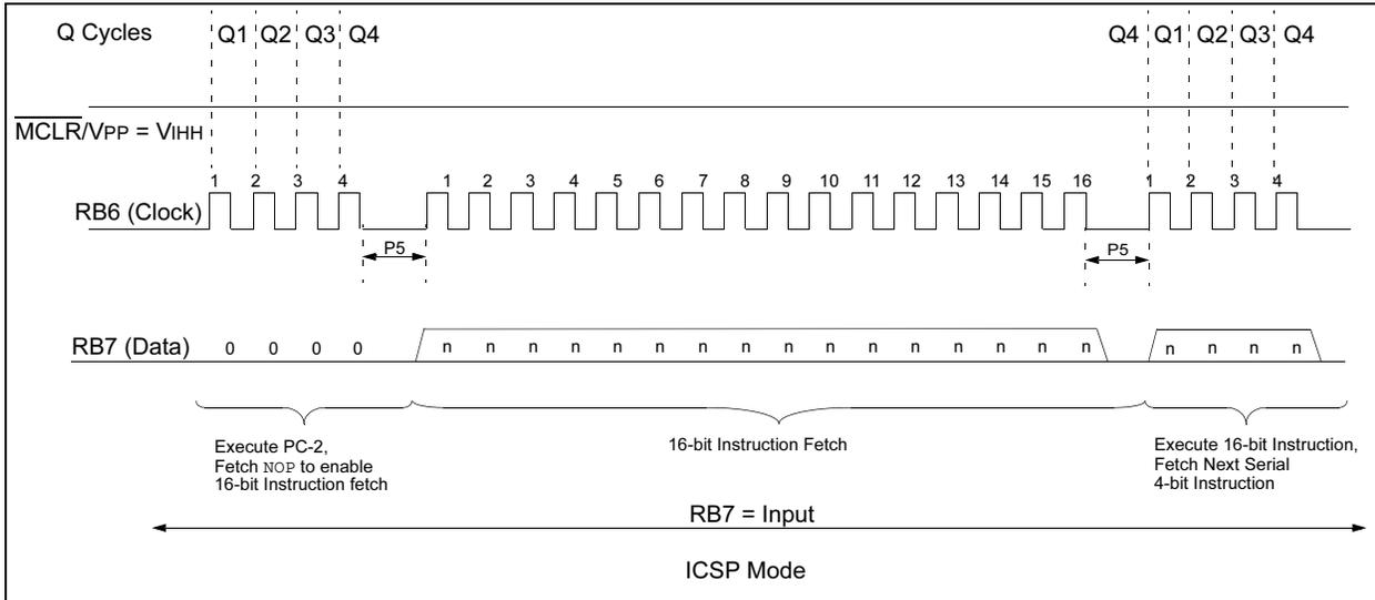
**FIGURE 2-3: 16-BIT, 1-CYCLE SERIAL INSTRUCTION FLOW AFTER RESET**
