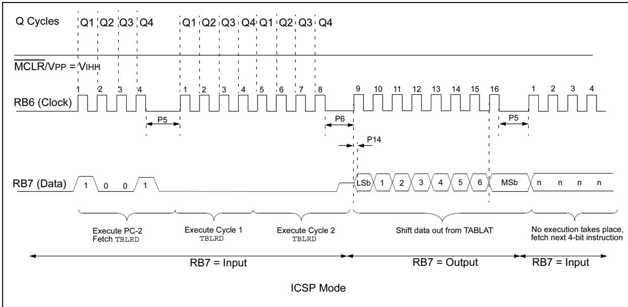
**FIGURE 2-13: TBLRD SERIAL INSTRUCTION FLOW AFTER RESET**
