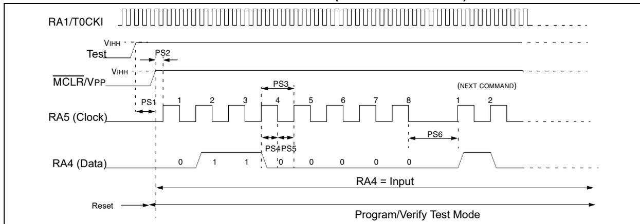
**FIGURE 7-3: LOAD ADDRESS COMMAND**
