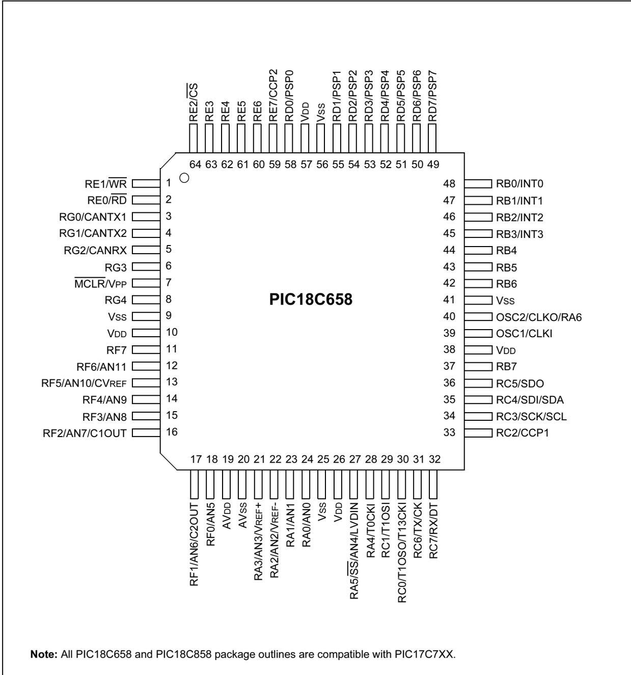
**FIGURE 1-5: PIC18C658 68-PIN PLCC DIAGRAM**
