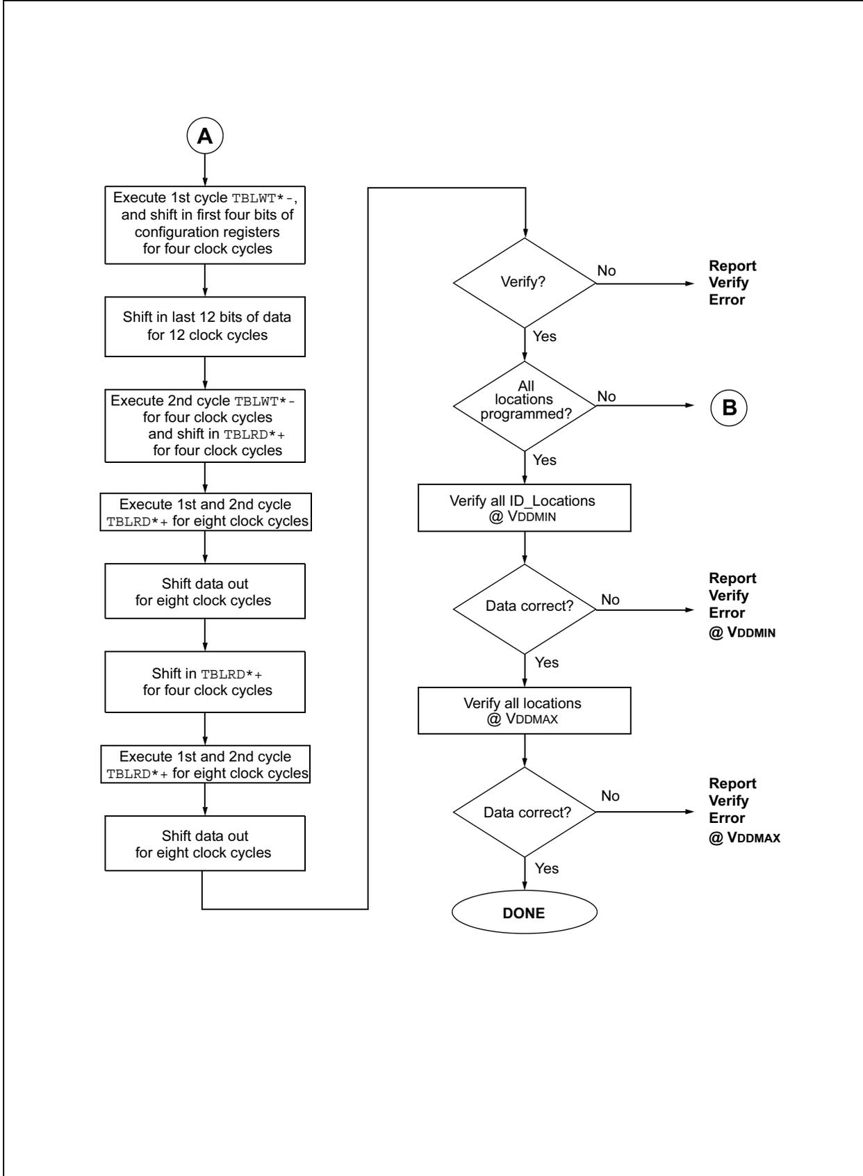
**FIGURE 2-24: DETAILED PROGRAMMING FLOW CHART – ID LOCATION**
