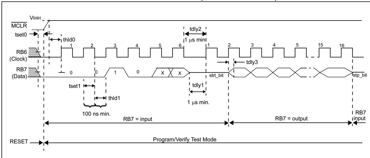
**FIGURE 6-3: INCREMENT ADDRESS COMMAND  $\overline{\text{MCLR}} = V_{\text{IH}}$  (PROGRAM/VERIFY)**
