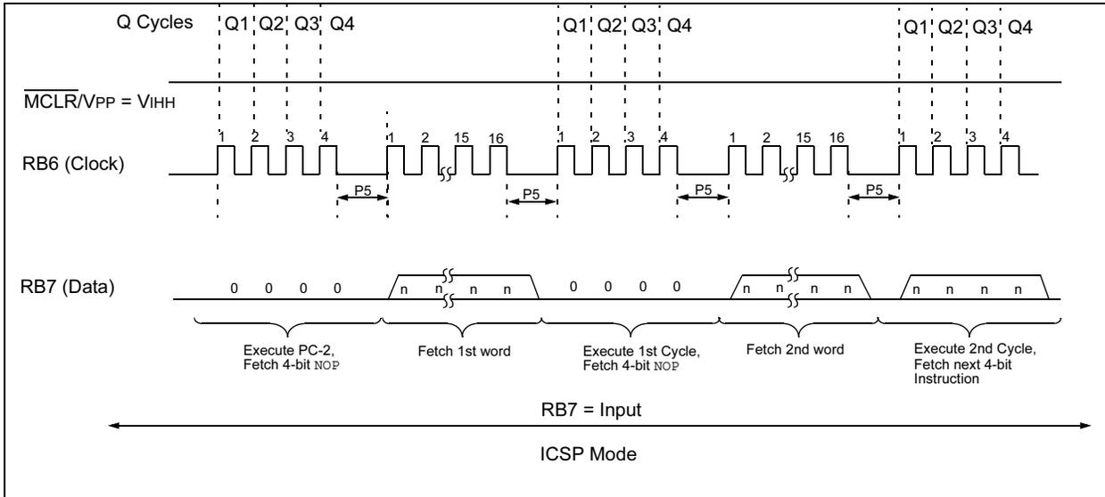
**FIGURE 2-7: 16-BIT, 2-CYCLE, 2-WORD SERIAL INSTRUCTION FLOW AFTER RESET**
