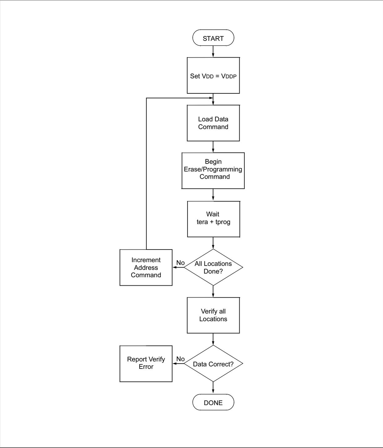
FIGURE 2-2: FLOW CHART – PIC16F87X PROGRAM MEMORY ( $4.5V \leq V_{DD} \leq 5.5V$ )
