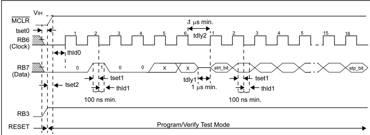
**FIGURE 6-5: READ DATA COMMAND  $\overline{\text{MCLR}} = V_{\text{DD}}$  (PROGRAM/VERIFY)**
