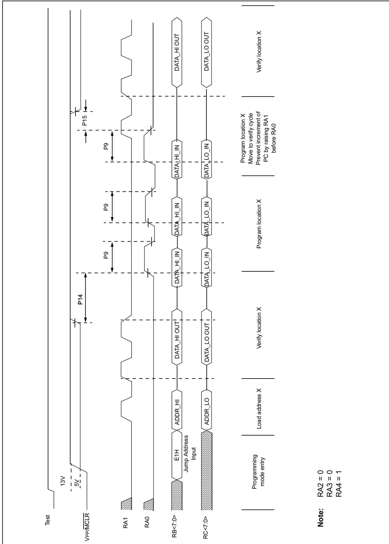
**FIGURE 6-3: PARALLEL MODE PROGRAMMING AND VERIFY TIMINGS III**
