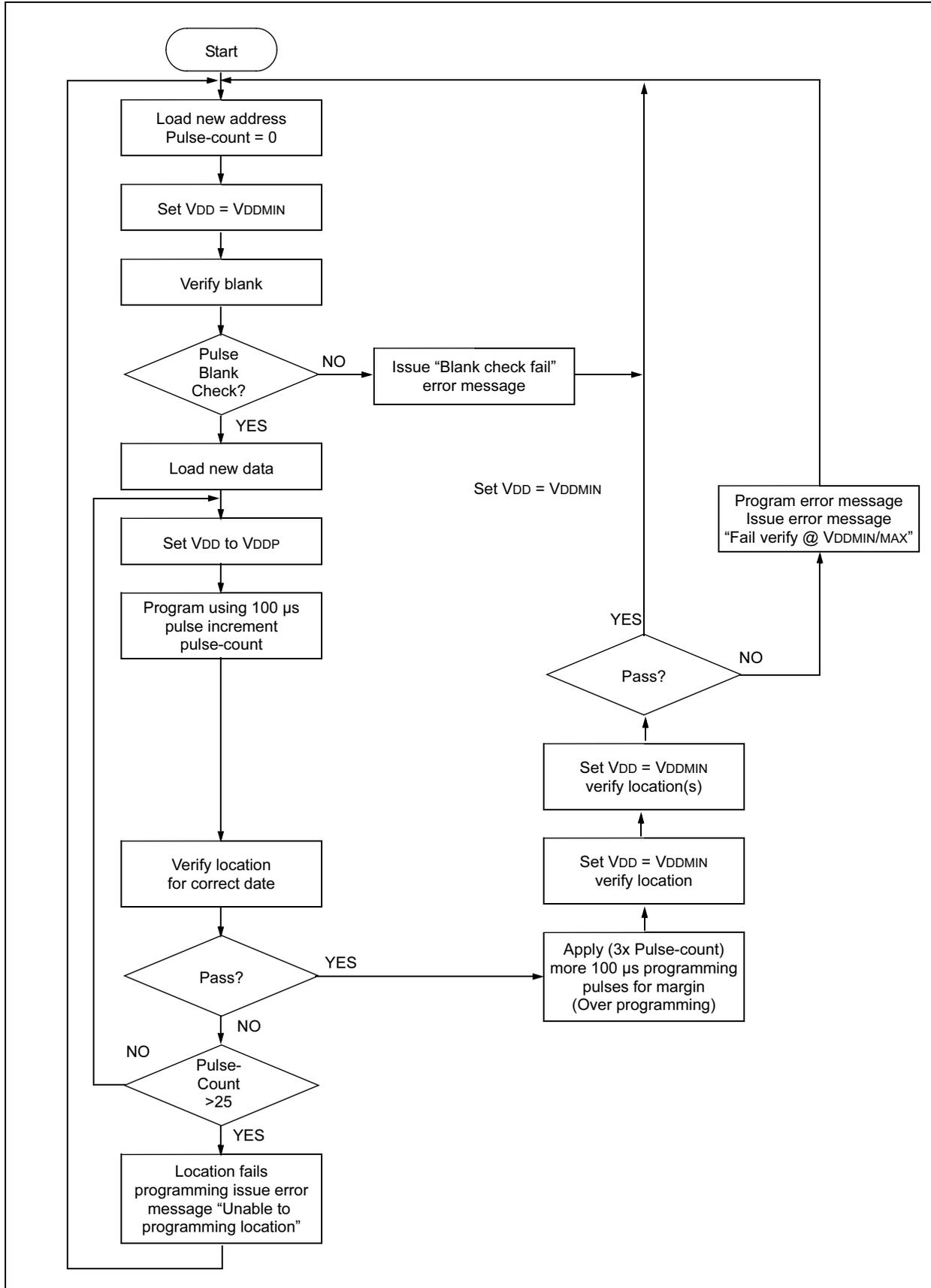
**FIGURE 3-3: RECOMMENDED PROGRAMMING ALGORITHM FOR CONFIGURATION WORDS**
