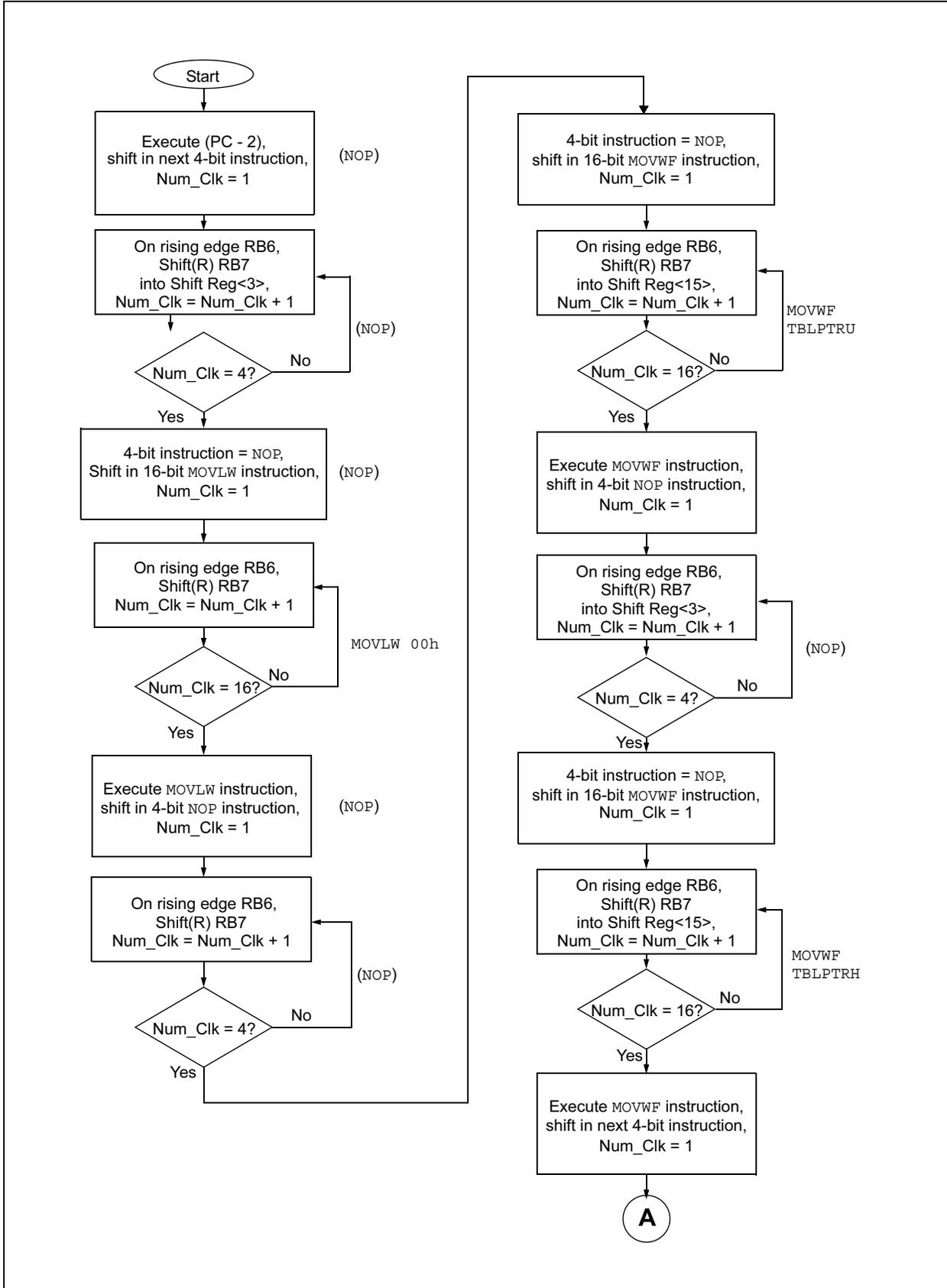
**FIGURE 2-16: RESET ADDRESS SERIAL INSTRUCTION SEQUENCE (CONTINUED)**
