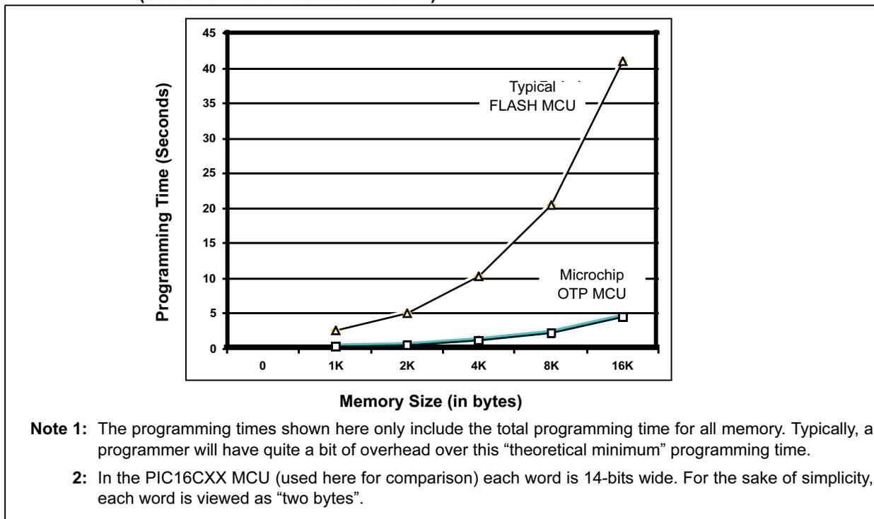
**FIGURE 2: PROGRAMMING TIME FOR FLASH AND OTP MCUS
