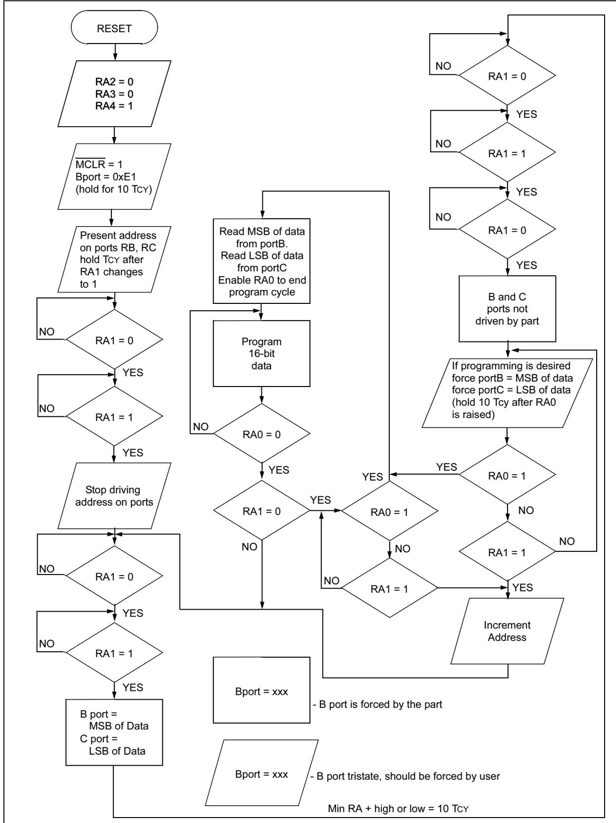
**FIGURE 3-2: RECOMMENDED PROGRAMMING ALGORITHM FOR USER EPROM**
