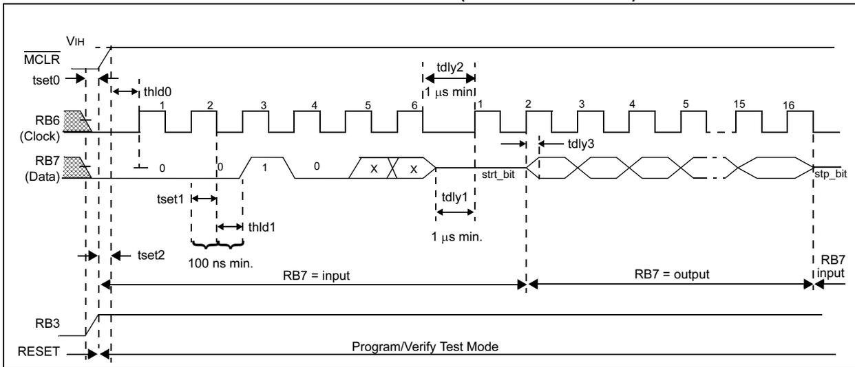
**FIGURE 6-6: INCREMENT ADDRESS COMMAND  $\overline{\text{MCLR}} = V_{\text{DD}}$  (PROGRAM/VERIFY)**
