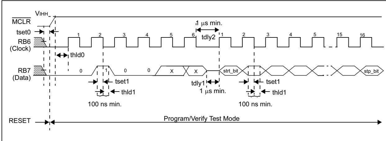
**FIGURE 6-2: READ DATA COMMAND  $\overline{\text{MCLR}} = V_{\text{IH}}$  (PROGRAM/VERIFY)**
