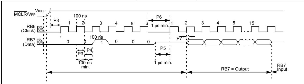
**FIGURE 4-3: INCREMENT ADDRESS COMMAND (PROGRAM/VERIFY)**
