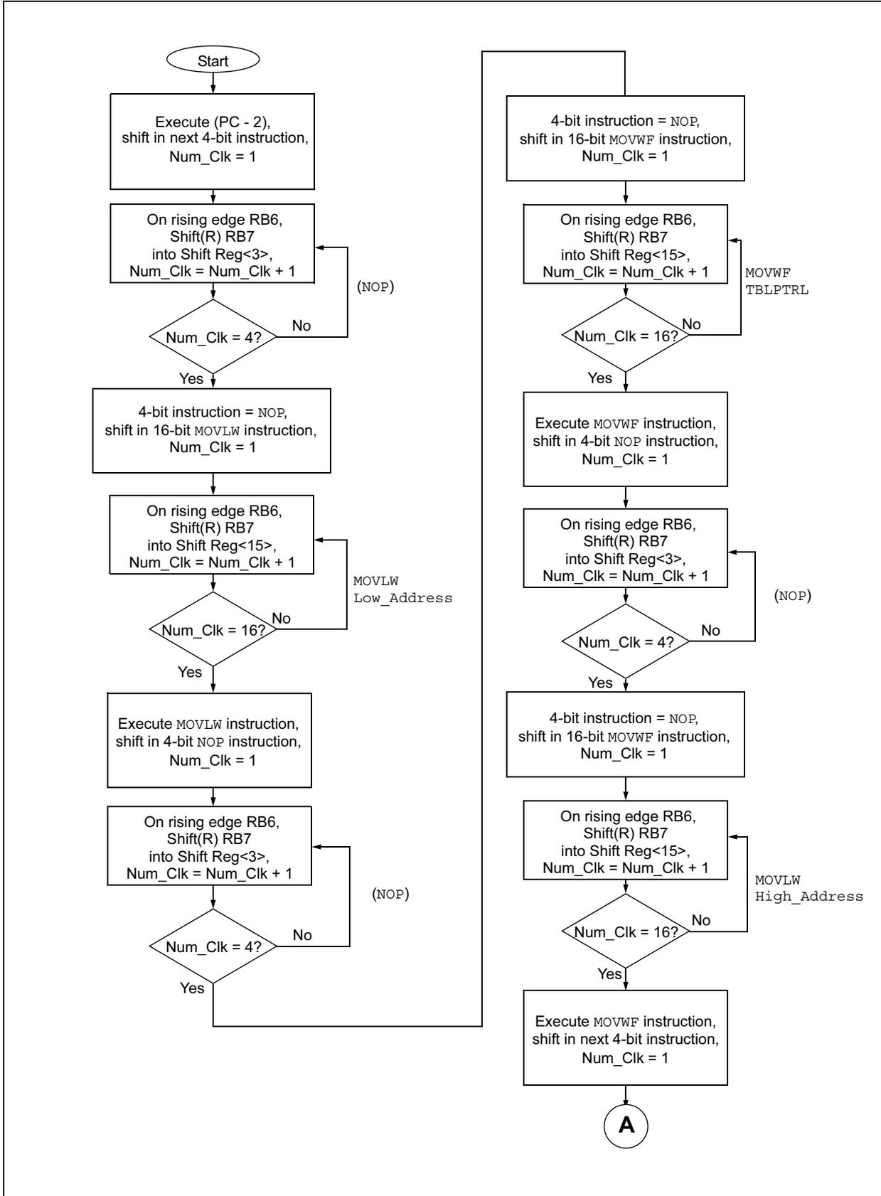
**FIGURE 2-18: LOAD ADDRESS SERIAL INSTRUCTION SEQUENCE (CONTINUED)**
