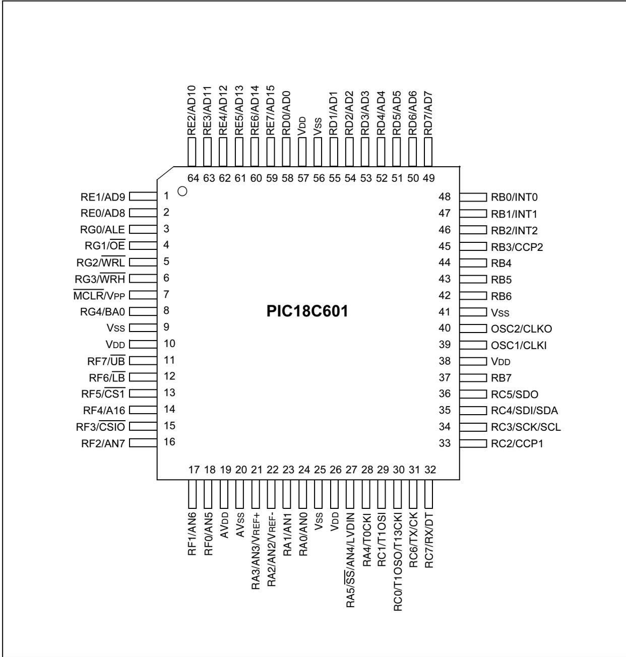
**FIGURE 1-9: PIC18C601 68-PIN PLCC DIAGRAM**
