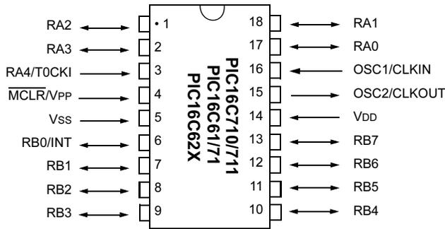
**300 mil. SDIP, SOIC, Windowed CERDIP, SSOP**
