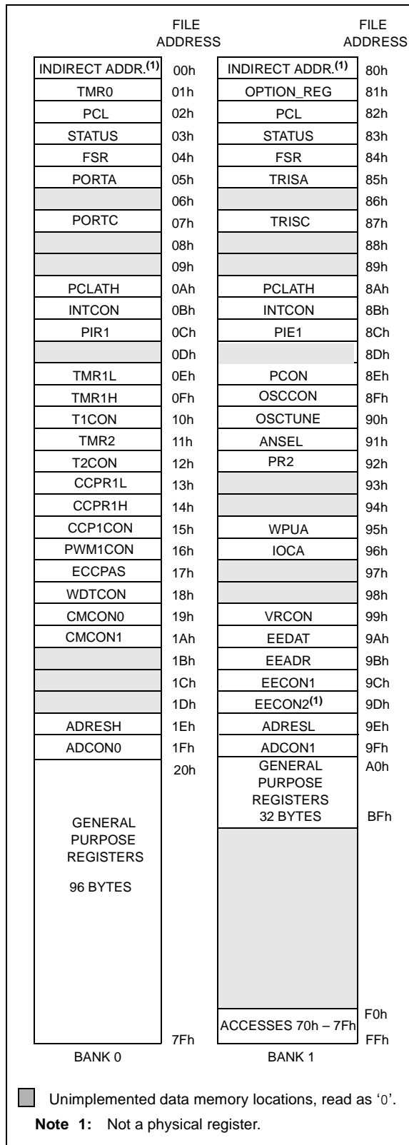
FIGURE 2-2: DATA MEMORY MAP OF THE PIC16F684
