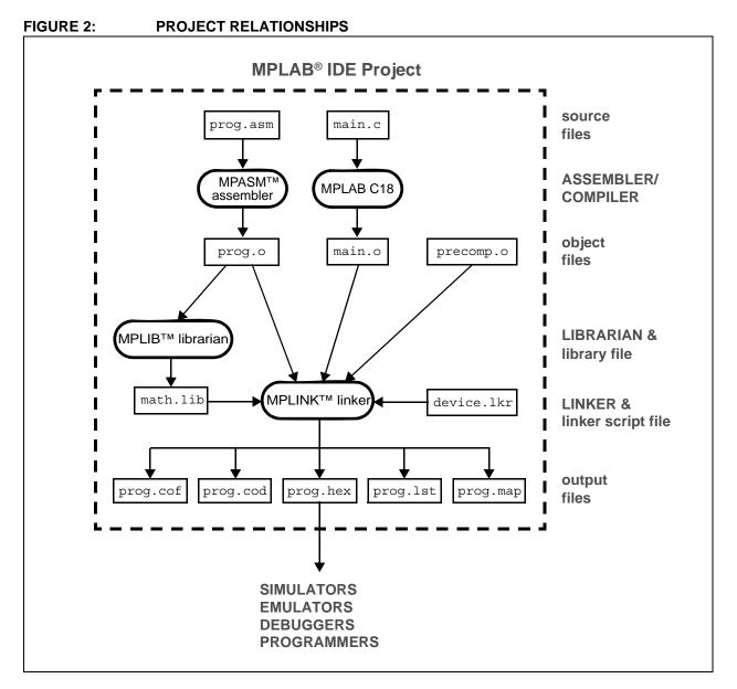
In this MPLAB IDE project, an assembly source file (prog.asm) is shown with its associated assembler (MPASM assembler). MPLAB IDE will use this information to generate the object file prog.o for input into the MPLINK object linker. For more information on the assembler, see the MPASM assembler documentation.
