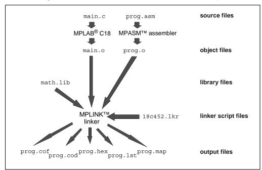
Below is a diagram of how the MPLINK linker works with other Microchip tools.
