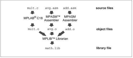
The librarian combines multiple input object modules, generated by the MPASM assembler or MPLAB C18 C compilers, into a single output library (.lib) file. Library files are used in conjunction with the MPLINK linker to produce executable code.
