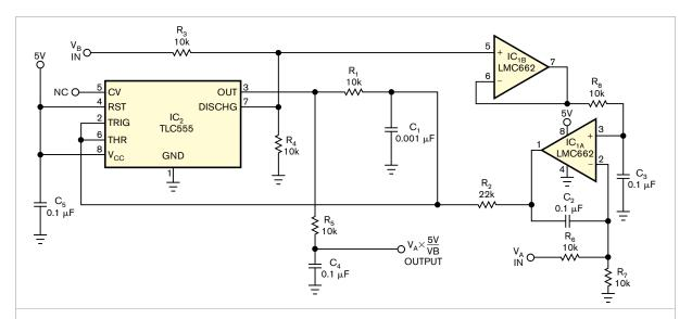
Figure 1 This low-cost pulse-width modulator performs analog division. Inputs  $V_A$  and  $V_B$  control this low-cost pulse-width modulator, and a lowpass filter follows it.
