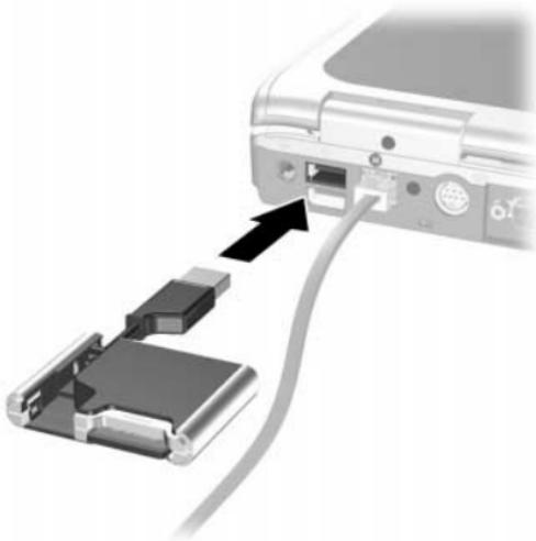
The status light on the Digital Drive turns on when the connection is successful. If the status light does not turn on, remove the Digital Drive from the USB port, then reinsert the USB connector.
