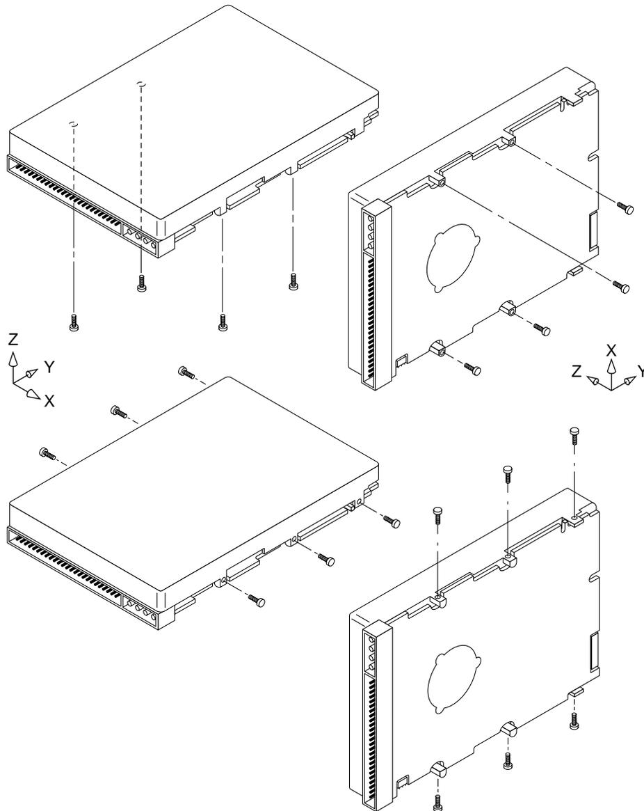
**Note.** Use four screws (two per side) when using the mounting holes located on the sides of the drive. See Section 8.4 when using the mounting holes located on the bottom of the drive.
