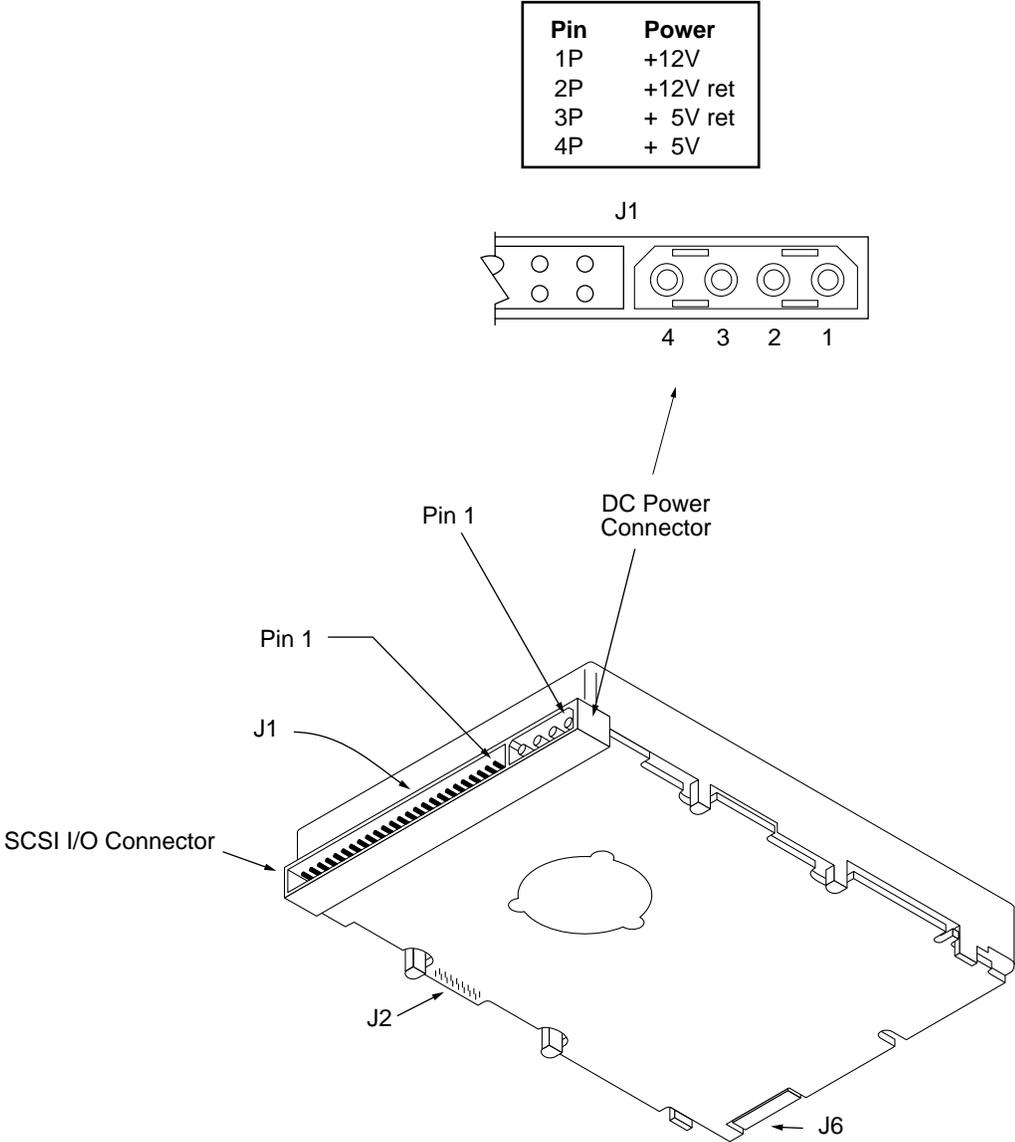
Figure 9a. Physical interface for "N" model drives
