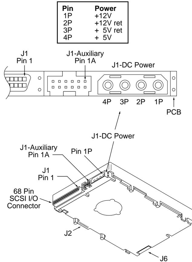
Figure 9b. Model “W” and “WD” drive physical interface (68 pin J1 SCSI I/O connector)
