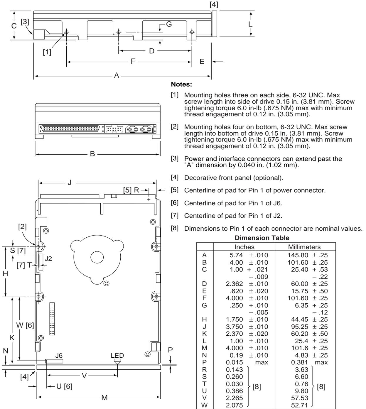
Figure 6b. Mounting configuration dimensions for models "W" and "WD"
