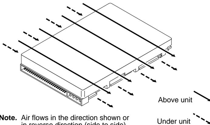
**Note.** Air flows in the direction shown or in reverse direction (side to side)
