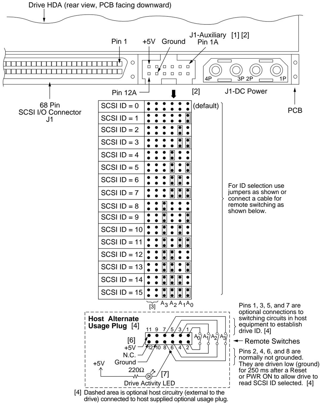
Figure 7c. Barracuda 4LP family drive ID select header J1-auxiliary for models “W” and “WD” (J1-Auxiliary Pins 1A - 12A)
