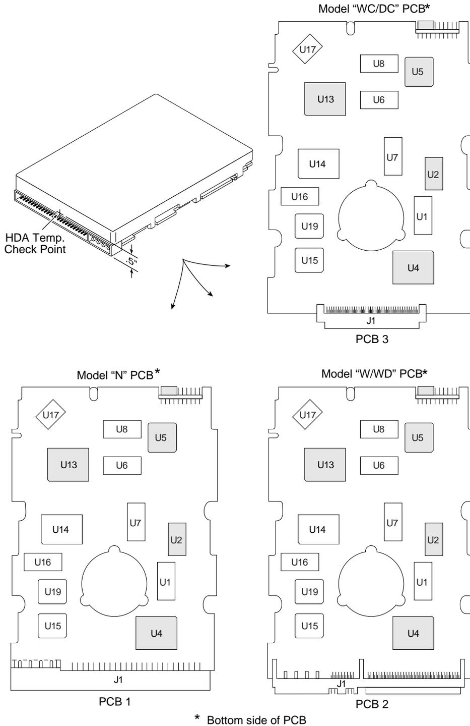
Figure 4. Locations of PCB components listed in Table 3
