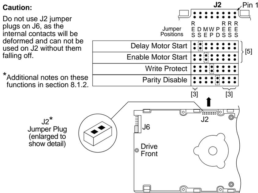
Figure 7e. Barracuda 4LP family drive option select header for models "WC" and "DC"
