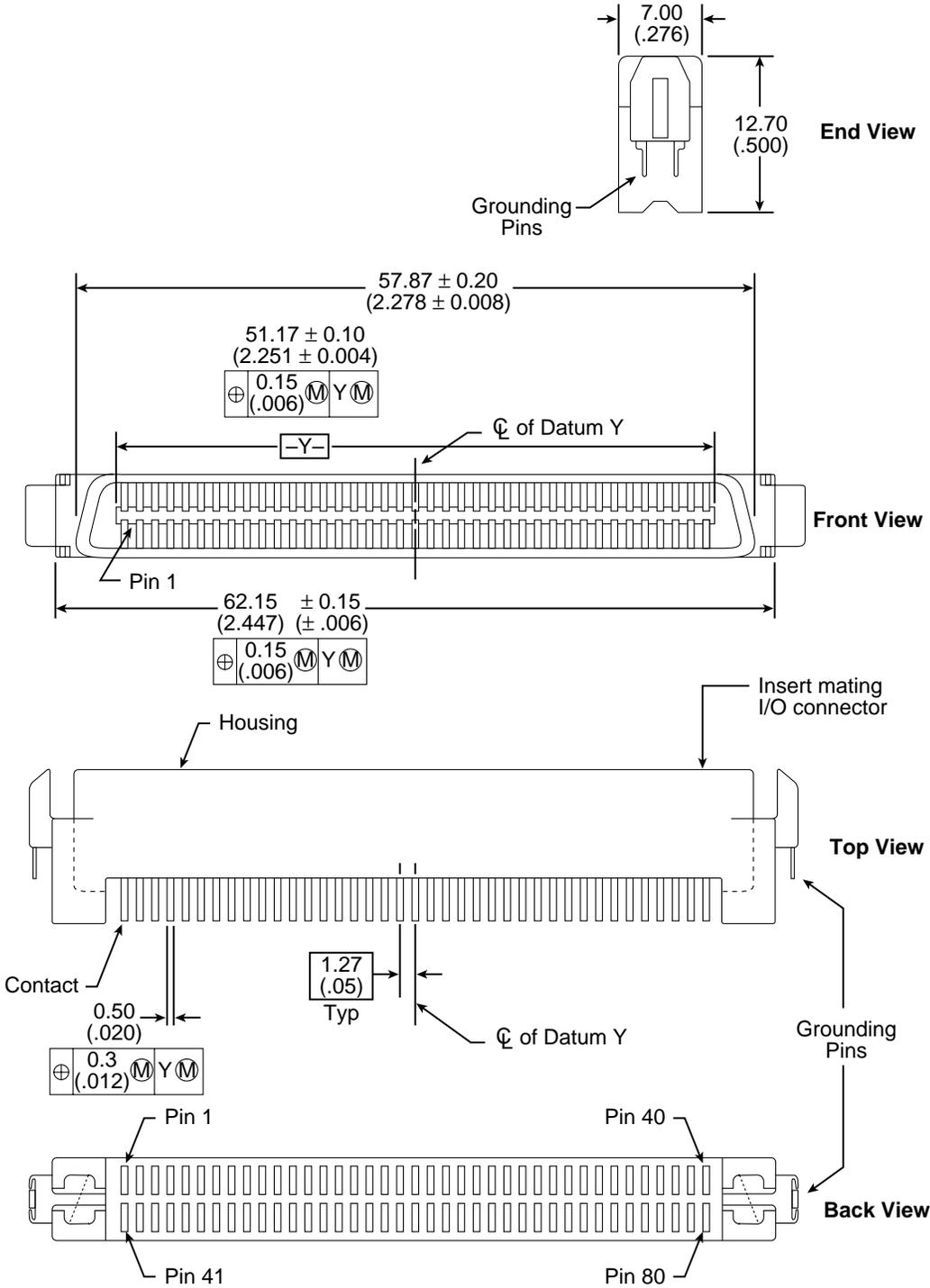
Figure 11c. Nonshielded 80 pin SCSI "SCA-2" connector, used on "WC" and "DC" models
