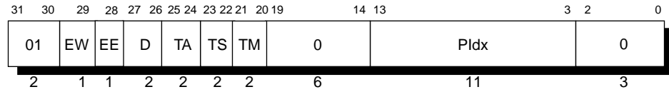
Figure 13-25 CacheErr Register Format for Primary Data Cache Errors
