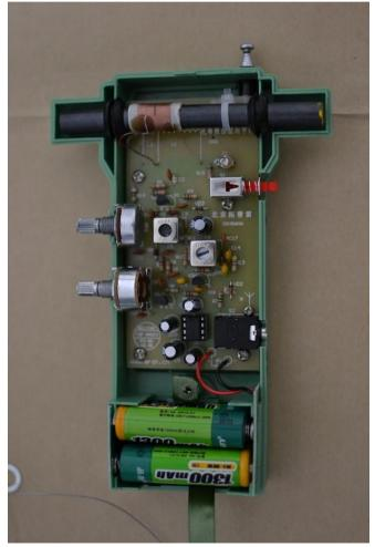
[ ] Place a transmitter nearby, and connect a dummy load. Adjust the RF power output to minimum (no bigger than 5 watts). Send CW signal and you should be able to hear from the ARDF receiver after fine tune. Follow the full manual instruction to send 3.53-MHz test signal, and adjust C1 to peak the signal. If not possible to peak the signal, you can adjust the location of the coil on the magnetic rod. Then, send 3.57-MHz test signal and you can turn T1 to peak the signal again.
