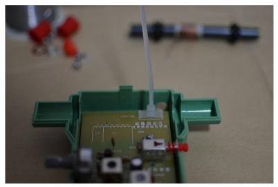
[ ] Bind the magnetic rod with the nylon strip, check the coil windings to the tap (with less turns on the left), adjust the location, and tighten.
