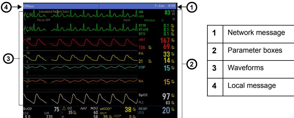
The standard Delta monitor provides five waveforms with adjacent parameter boxes. Kappa provides four waveforms with adjacent parameter boxes. Delta XL provides six waveforms with adjacent parameter boxes. Channels can be added to display up to eight waveforms. The bottom channel can be used to display additional parameter boxes (see “Bottom Channel” on page 2-6).
