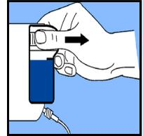
4. Aspirate the water trap contents into syringe.
