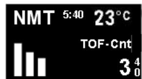
You can set TOF-count alarm limits and alarm recordings in the Alarm Limits table (see chapter 5, Alarms).
