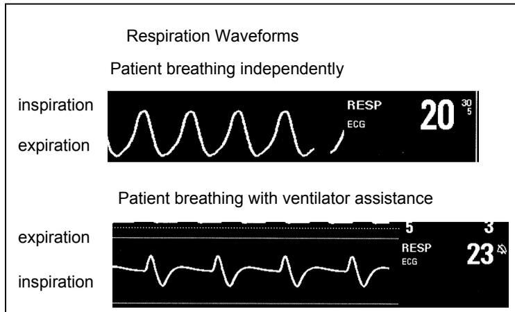
In the RESP parameter box, a lung symbol (☁) blinks whenever a breath is detected. The display of respiration alarms, alarm limits, and parameter values follows the standard display of other parameters.
