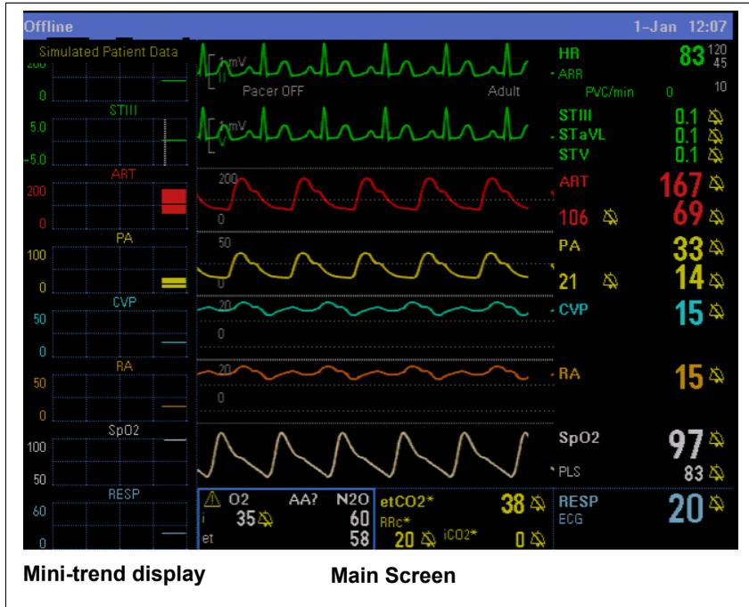
**NOTE:** You can only select one parameter for the mini trend display from a parameter box that contains multiple parameters.
