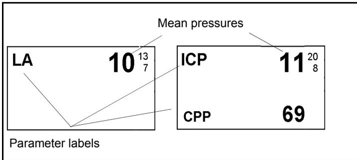
The CPP parameter is calculated and displayed whenever the ICP and ART parameters are monitored simultaneously ( $CPP = ART_{\text{mean}} - ICP$ ). CPP/ CPP2/ CPP3/ CPP4 is displayed in the bottom of the ICP/ ICP2 / ICP3/ ICP4 parameter box.
