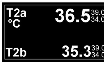
When monitoring temperature using the Hemo2, Hemo4 pod, or the MPod – Quad Hemo, temperature values are further identified according to where they are connected to the monitor. The temperature value corresponding to the device hooked up to the Aux/Hemo2 PodCom connector is labeled T2a or T2b, while the temperature
