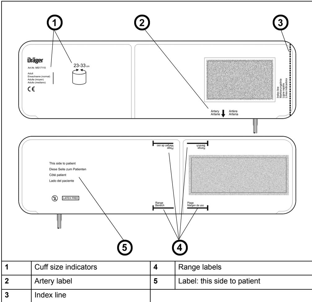
To avoid kinks in the hose, center the cuff bladder on the artery so that the hose is to the left or to the right of the artery. Ideally, blood pressure measurements should be taken with the cuff positioned at heart level. If the cuff is not placed at heart level, adjust the displayed systolic and diastolic readings +8mmHg for each 10cm above the heart and -8mmHg for each 10cm below the heart.
