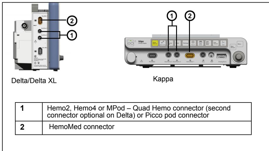
2. Connect the other end of the cable into the hemodynamic pod connection port.
