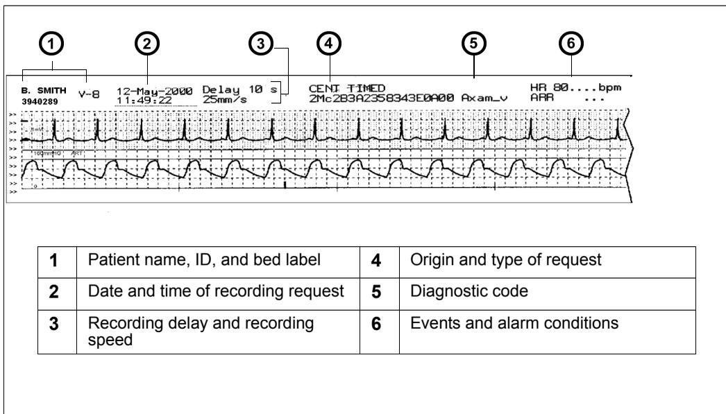
**NOTE:** Values and alarm off indicators active at the time of the recording request are printed after the recording header for each parameter (if appropriate).
