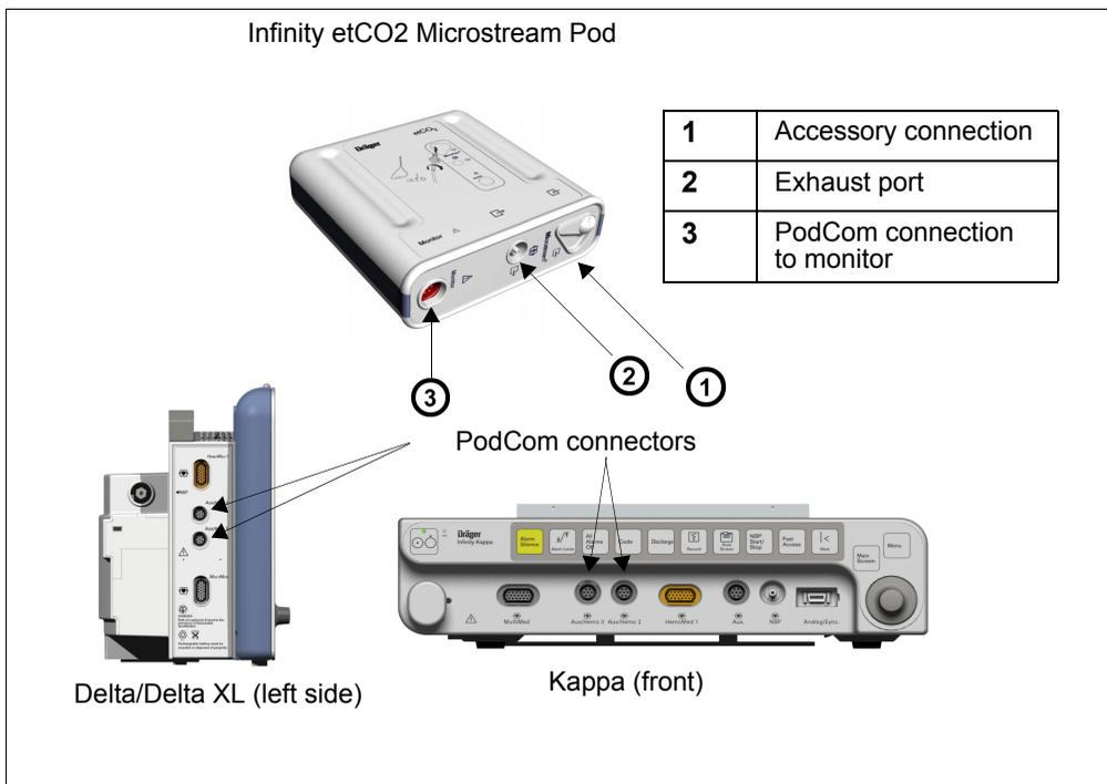
1. Plug one end of the connecting cable into either of the two PodCom connectors on the monitor (the second PodCom connector is optional on the Delta).
