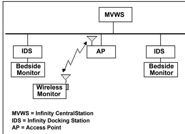
If a wireless monitor loses contact with all access points and wireless transmission is interrupted (for example, you remove the wireless card or the monitor is out of range), the network generates an offline message and the monitor operates as a standalone device.
