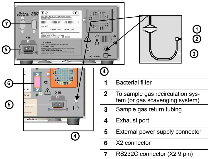
4. Connect one end of the Scio connecting cable to the X2 connector at the rear of the module and the other end to the Delta/Delta XL/Kappa monitor or to the IDS (see “Cable Connections” on page 23-9). If you are using a breakout box, connect the end to the connector on the breakout box.
