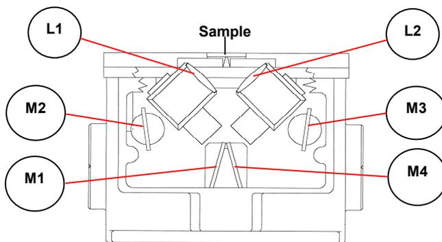
**Fig 11. Optical Components in the Golden Gate™ Optical Unit Related to the Beam Passage for L to R or R to L Direction Spectrometers**
