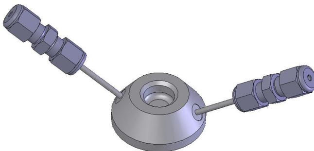
**Fig 23. Micro Reaction Flow Cell Anvil GS10568**
