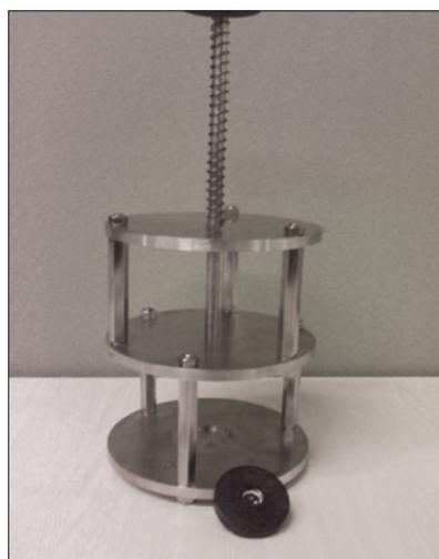
Figure 3. Powder sample press with sample holder.
