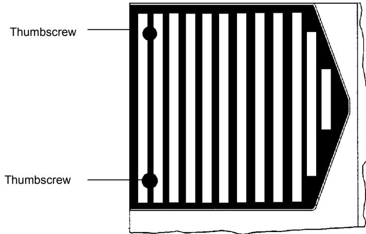
**Figure 19 Lamp baffle**
