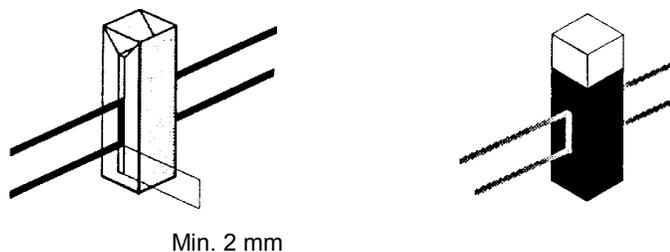
**Figure 11 Correct Alignment of the Radiation Beam in the Cell Sample Area**
