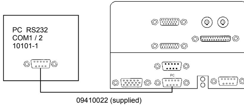
Figure 8 Connecting the PC to the spectrometer
