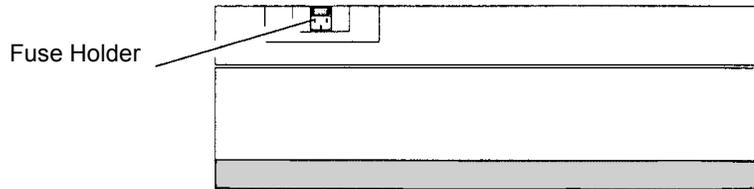
**Figure 26 Rear view, fuse holder**
