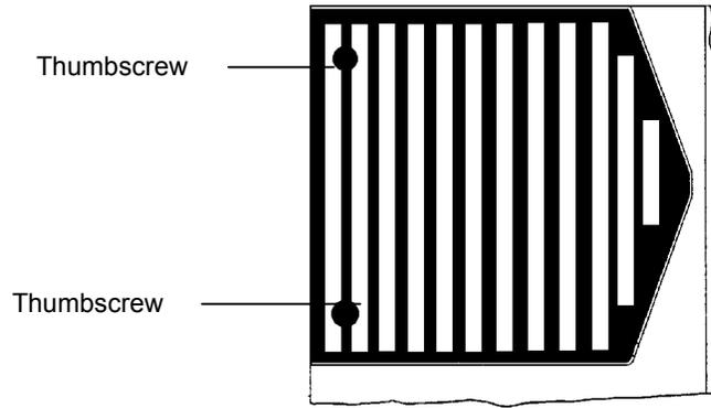
**Figure 22 Lamp baffle**
