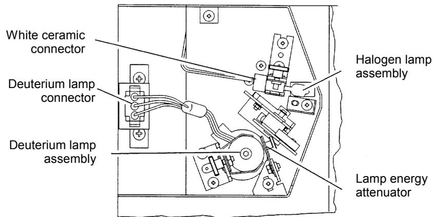
**Figure 17 Inside the Lamp Compartment (Baffle removed)**
