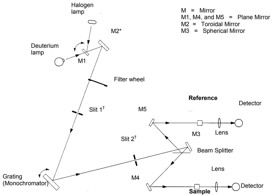
**Figure 6 Optical Path for Lambda 25, 35, 45**
