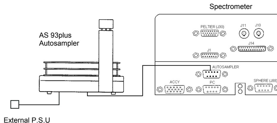
**Figure 15 Autosampler electrical connection**
