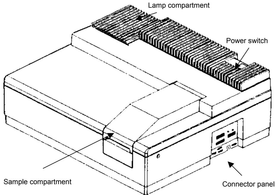
**Figure 5** Lambda 25, 35, 45 Spectrometer Features
