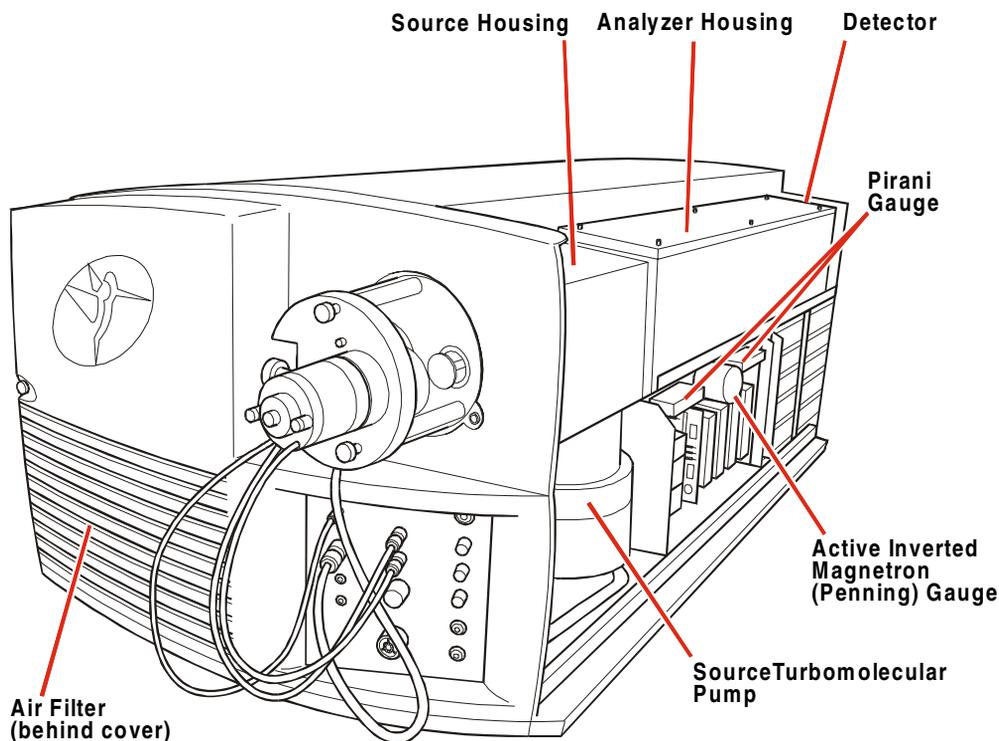
Figure 1-17 Main Internal Mechanical Components
