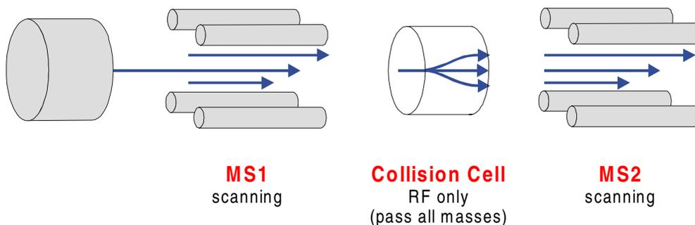
Figure 1-9 Constant Neutral Loss Spectrum
