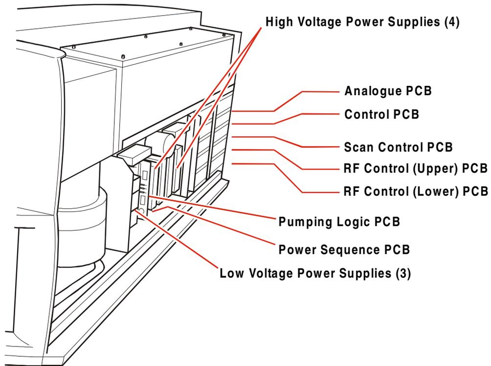
Figure 1-15 Internal Layout of Electronics
