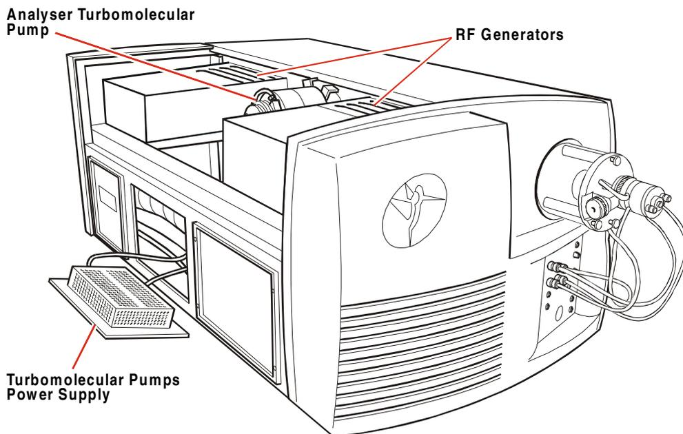
Figure 1-16 Main Electronics Modules
