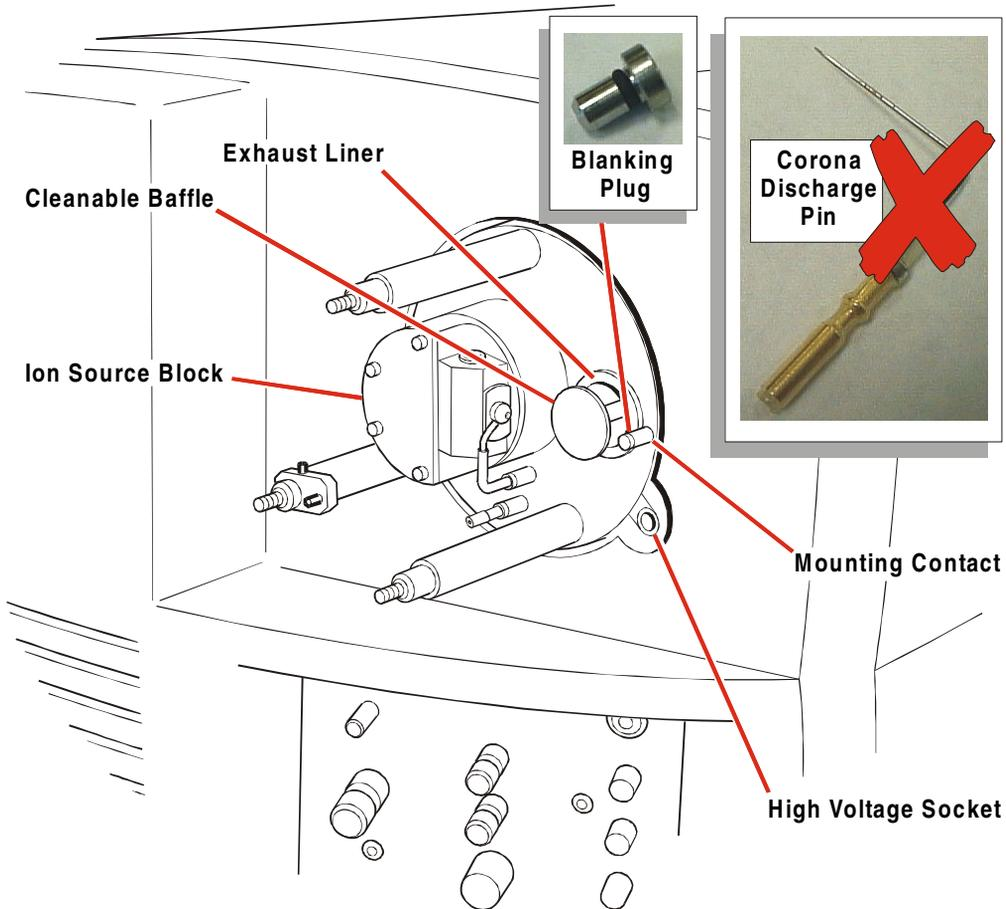
Figure 2-6 Replacing the Corona Discharge Pin For ESI
