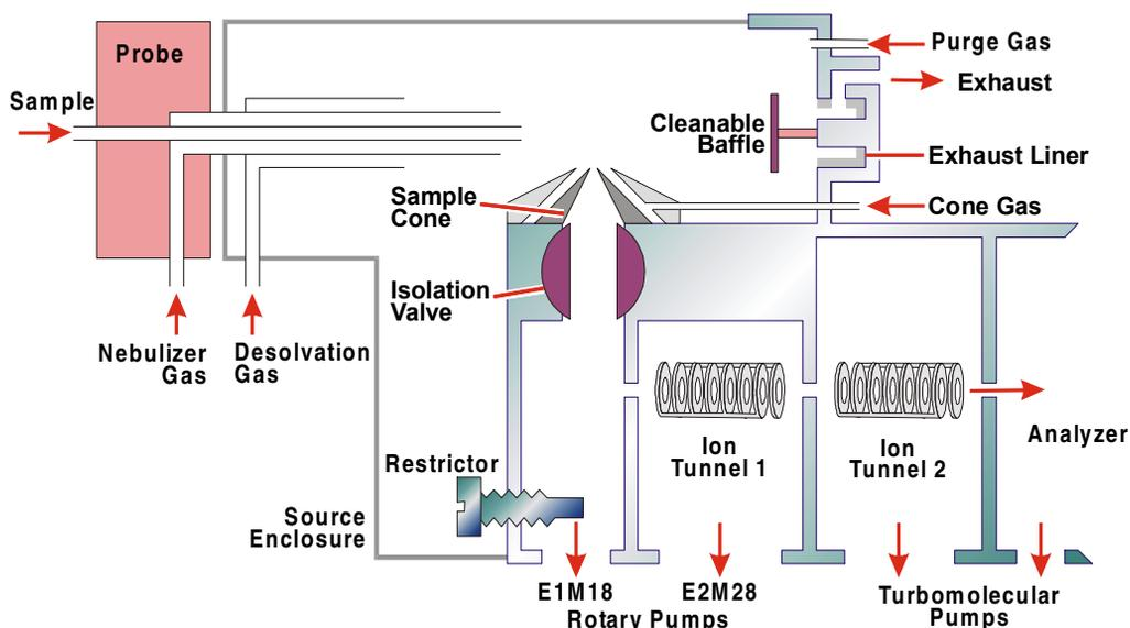
Figure 6-1 ElectroSpray Ionization
