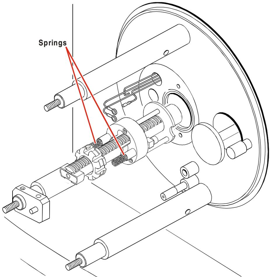
Figure 8-9 Ion Tunnel Assembly Springs
