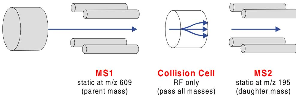
Figure 1-7 Multiple Reaction Monitoring
