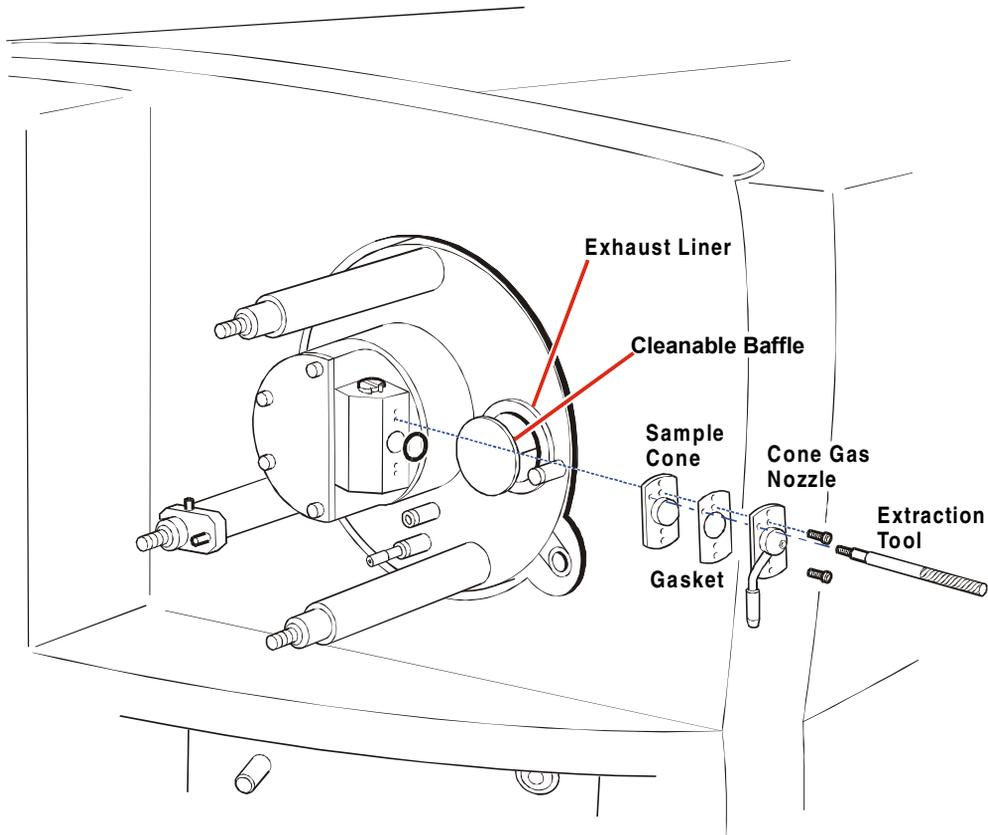
Figure 8-4 Sample Cone Removal
