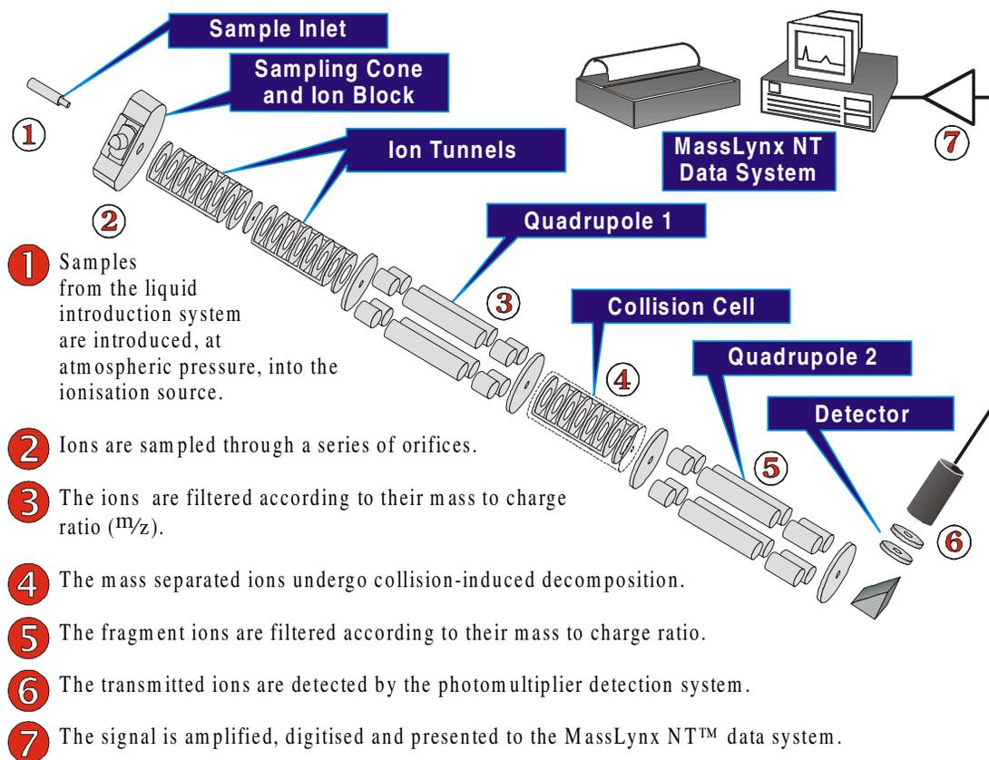
Figure 1-1 Micromass Quattro Ultima Pt Ion Optics
