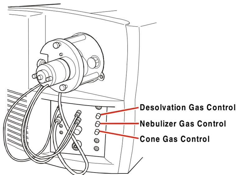
Figure 6-8 Gas Flow Controls
