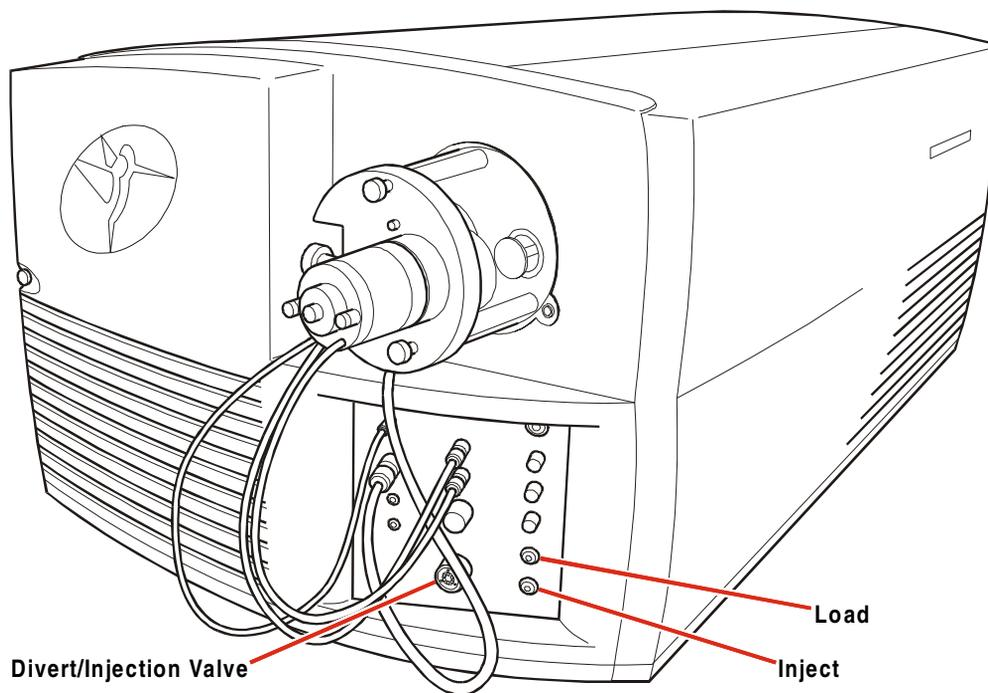
Figure 1-12 Divert/Injection Valve
