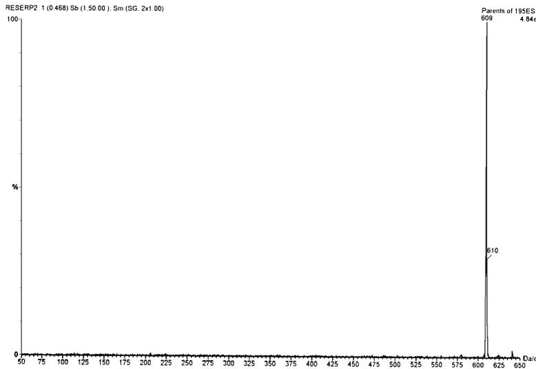
Figure 1-6 MS-MS Mode - Parent Ion Spectrum Example
