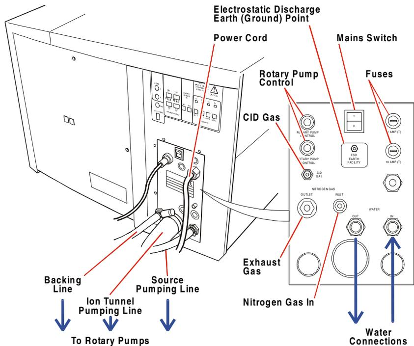
Figure 1-14 Rear Panel Connections
