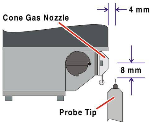
Figure 6-7 Probe Adjustment
