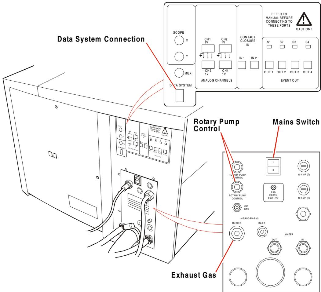
Figure 2-3 Rear Exhaust and Peripheral Connections
