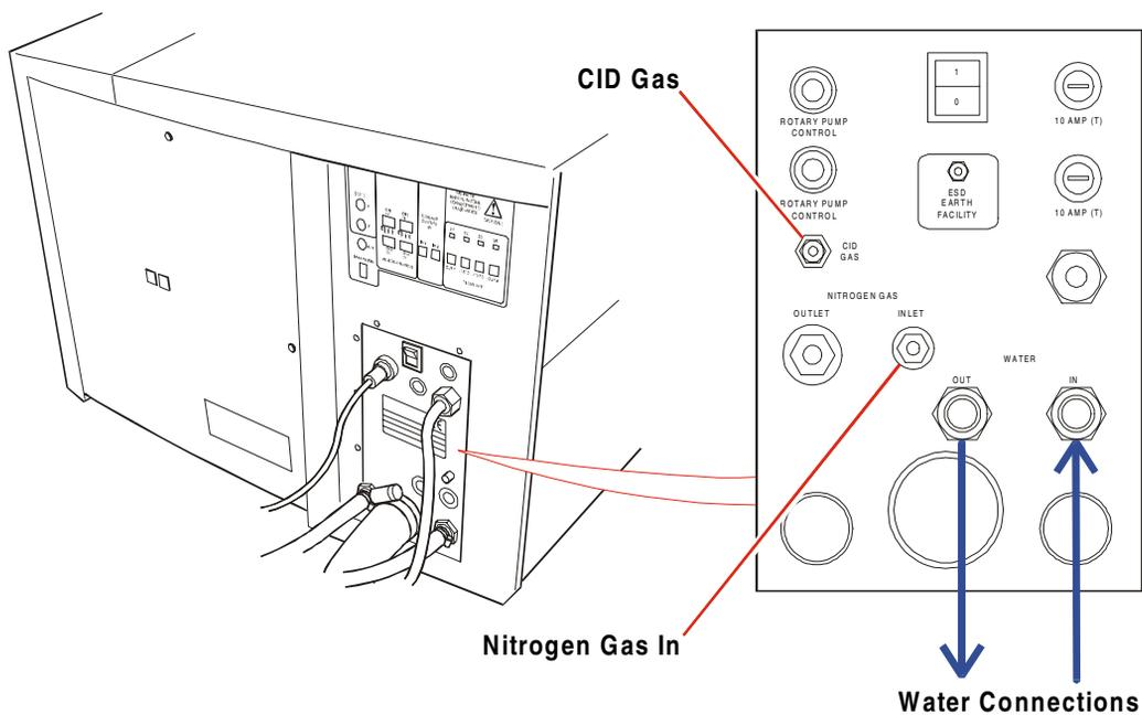
Figure 2-2 Gas/Water Connections
