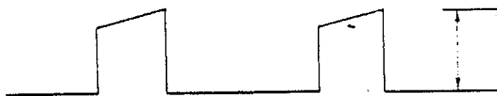
Fig. 5-1 Primary voltage characteristics of the DC-DC converter
