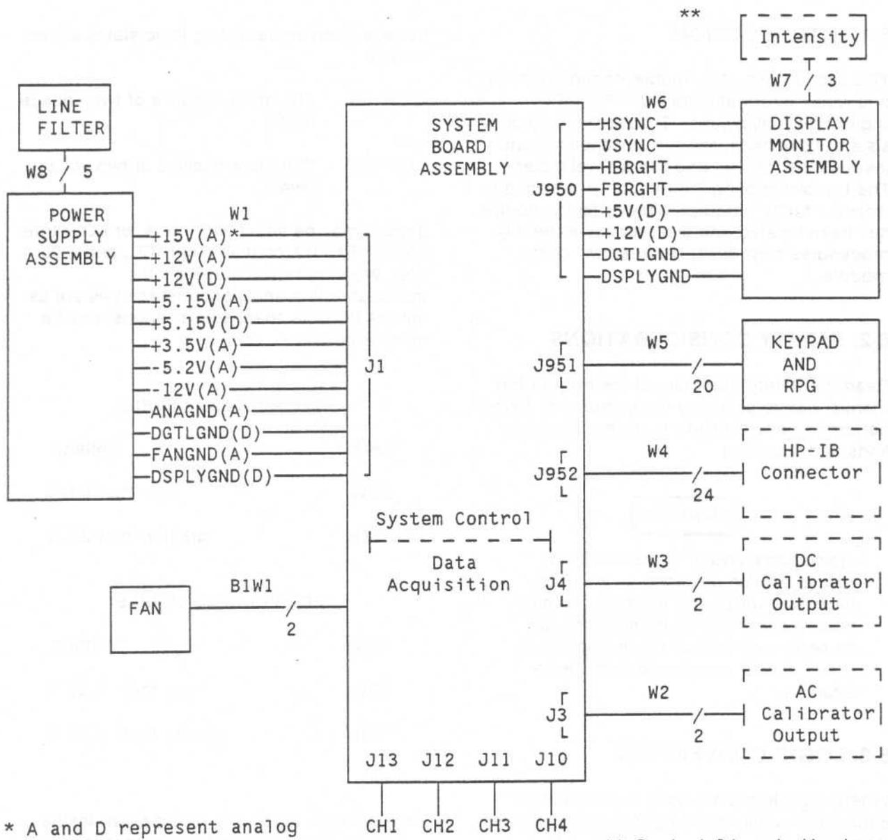
\* A and D represent analog and digital voltages from the power supply. Analog voltages are routed mainly to data acquisition section of the system board.
