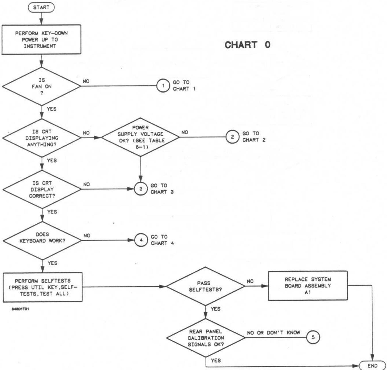
Figure 6-4. General Trouble Isolation Flowchart for HP 54501A
