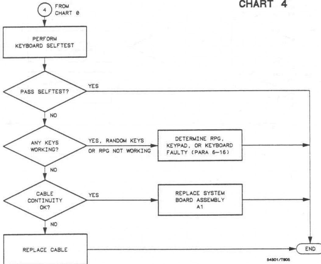
Figure 6-8. Trouble Isolation Flowchart for HP 54501A Keyboard
