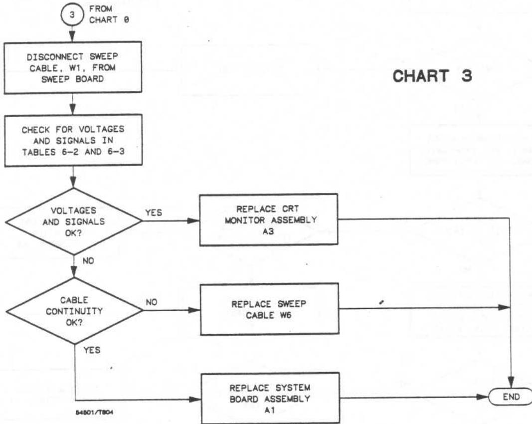
Figure 6-7. Trouble Isolation Flowchart for HP 54501A CRT Monitor
