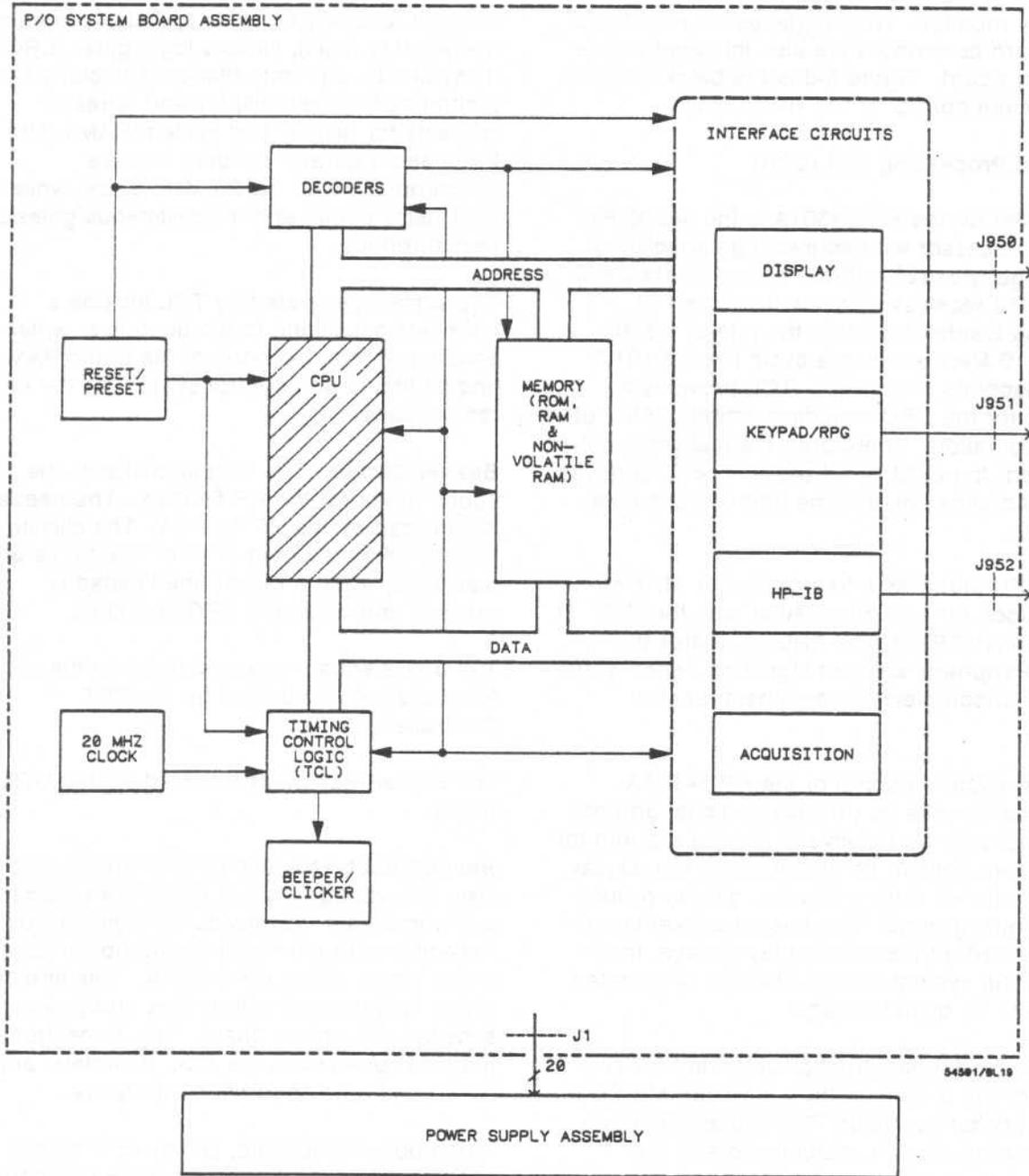
Figure 6-3. HP 54501A System Control Block Diagram
