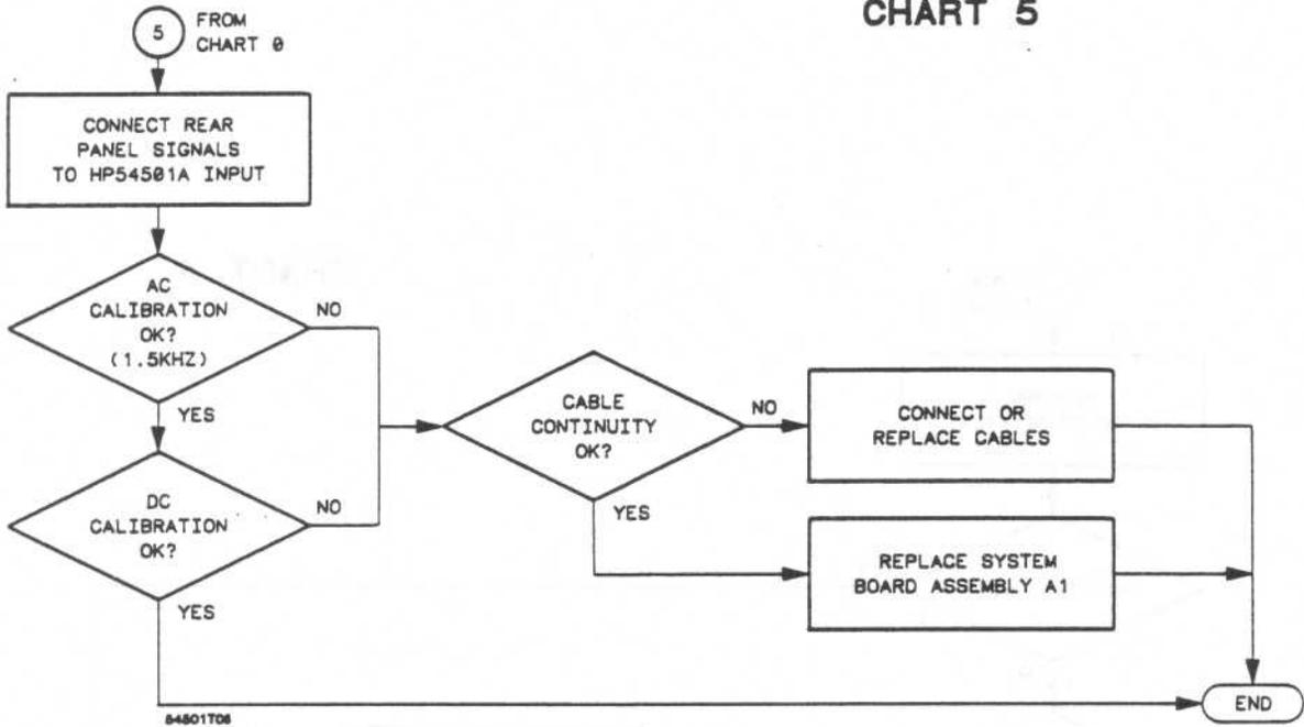
Figure 6-9. Trouble Isolation Flowchart for HP 54501A Calibration Signals
