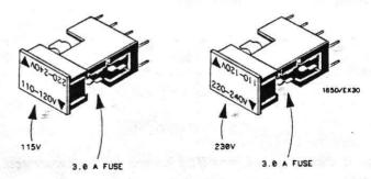
Figure 2-4. Checking for the Correct Fuse
