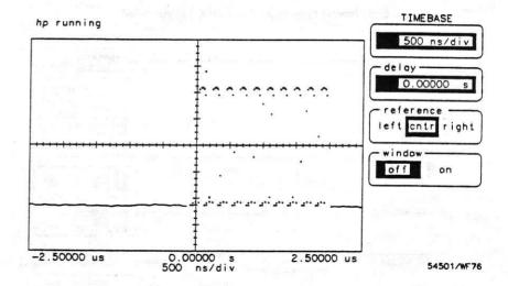
Figure 6-14. Ten Burst Pulse w/Stable Trigger
