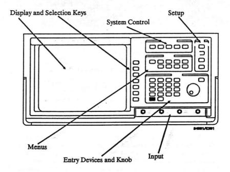
Figure 3-1. HP 54501A Front Panel
