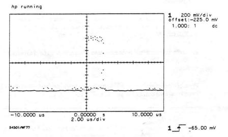
Figure 6-13. Ten Burst Pulse after AUTOSCALE
