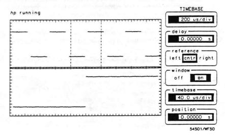
Figure 4-3. Input Signal with Window Turned On
