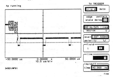
Figure 6-20. Trigger on Field 2, Line 1
