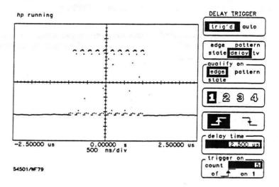
Figure 6-15. Ten Burst Pulse Triggered on Pulse 5
