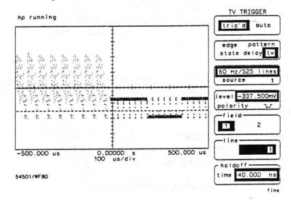
Figure 6-17. Trigger at Field 1, Line 1
