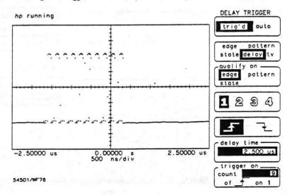
Figure 6-16. Ten Burst Pulse Triggered on Pulse 9
