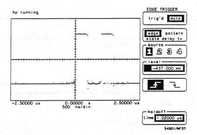
Figure 6-4. Two-Burst Pulse w/Stable Trigger
