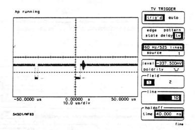
Figure 6-18. Trigger on Field 1, Line 10
