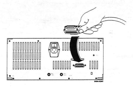
Figure 2-7. Connecting External Equipment
