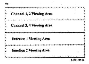
Figure 9-3. Dual Screen w/Function On
