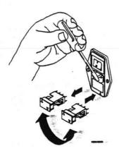
Figure 2-3. Selecting Line Voltage
