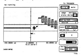
Figure 6-19. Trigger on Field 1, Line 21
