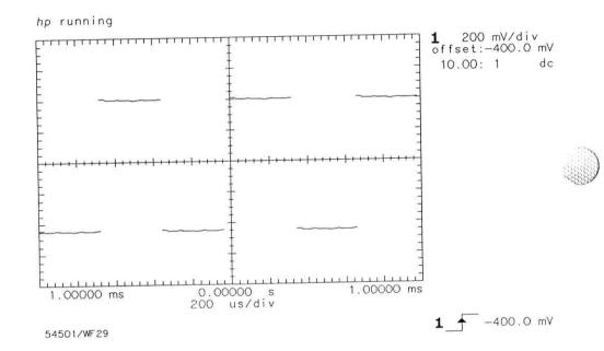
The channel settings and trigger information are displayed along the right edge of the display.
