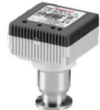
The Active Linear Convection Vacuum Gauge has a wide measuring range from 1333 to  $3 \times 10^{-4}$  mbar ( $1000$  to  $2.3 \times 10^{-4}$  Torr). The use of convection technology ensures accuracy and sensitivity are maintained to the top of the pressure range compared to conventional Pirani gauges, which lose accuracy above 100 mbar. The gauge is compact and may be mounted in any orientation, simplifying installation where space is limited.
