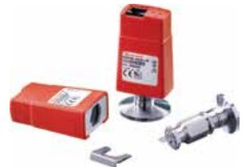
APG100 series Active Pirani vacuum gauges are available in 2 models. The APG100-XM is the standard model and measures to 10<sup>-3</sup> mbar, the APG100-XLC is a corrosion resistant version with measurement to 10<sup>-4</sup> mbar. Both gauges feature compact size for easy installation, a linear output and a replaceable sensor tube. These gauges are compatible with all Edwards TIC instrument controllers and other Active gauge controllers and displays.
