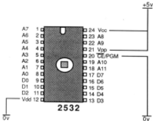
*Note: A bar above the pin designation indicates that the input is active when 'low'. See glossary of terms for an explanation of pin functions.*
