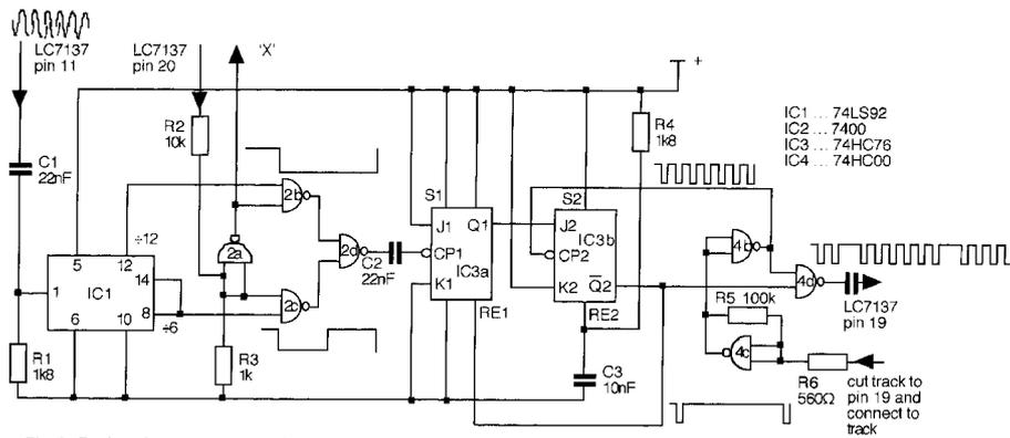
Fig. 1 Basic pulse blanking circuit
