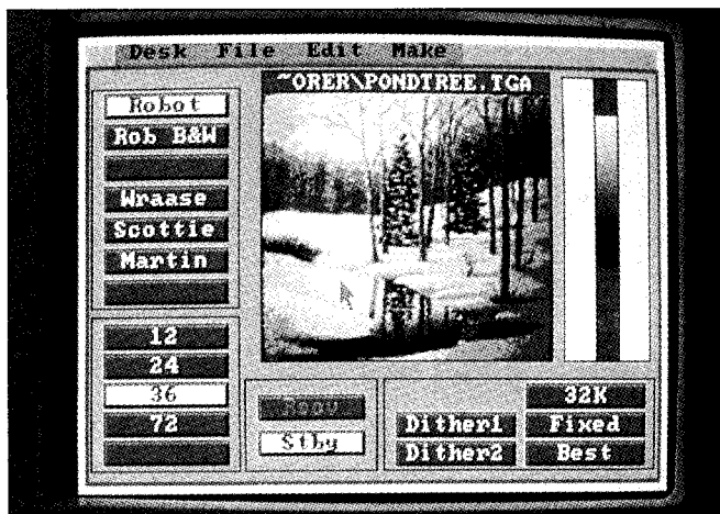
Figure 1—The Explorer's main menu. The top-left box displays the reception modes. Below that the mode variants of the selected mode are shown. At the far right side is a tuning bar that provides a real-time spectral display of the incoming signal and helps you zero-in on the frequency.
