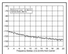
Figure 5—Worst-case tested spectral display of the IC-746 transmitter output during composite-noise testing on VHF. Power output is 100 W at 144.020 MHz. The carrier, off the left edge of the plot, is not shown. The plot shows composite transmitted noise 2 to 22 kHz from the carrier.
