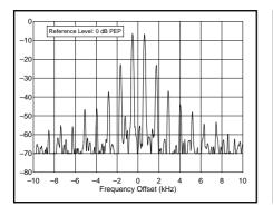
Figure 1—Worst-case spectral display of the IC-746 transmitter during two-tone intermodulation distortion (IMD) testing on HF. The worst-case third-order product is approximately 23 db below PEP output, and the worst-case fifth-order product is approximately 37 dB down. The transmitter was being operated at 100 W output at 28.350 MHz.
