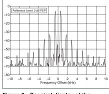
Figure 2—Spectral display of the IC-756PRO transmitter during two-tone intermodulation distortion (IMD) testing on 6 meters. The third-order product is approximately 34 dB below PEP output, and the fifth-order is approximately 40 dB down. The transmitter was being operated at 100 W output at 50.200 MHz.
