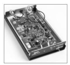
Figure 6—Inside the Ten-Tec 1210 10- to 2-meter transverter. Nearly all the unit's components are mounted on a single  $4 \times 5^{1}/_{2}$ -inch glass-epoxy PC board.
