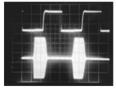
Figure 3—CW keying waveform for the IC-756PRO showing the first two dits in full-break-in (QSK) mode. The equivalent keying speed is 60 WPM. The upper trace is the actual key closure; the lower trace is the RF envelope. Horizontal divisions are 10 ms. The transceiver was being operated at 100 W output at 14.2 MHz. Note that both dits are somewhat shortened. Only the first dit is shortened in semi-break-in mode.
