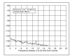
Figure 4—Worst-case tested HF spectral display of the IC-756PRO transmitter output during composite-noise testing at 14 MHz. Power output is 100 W. The carrier, off the left edge of the plot, is not shown. This plot shows composite transmitted noise 2 to 22 kHz from the carrier.
