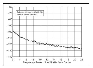
Figure 5—Spectral display of the unmodified IC-756 transmitter output during composite-noise testing at 50.2 MHz. Power output is 100 W. The carrier, off the left edge of the plot, is not shown. This plot shows composite transmitted noise 2 to 22 kHz from the carrier.
