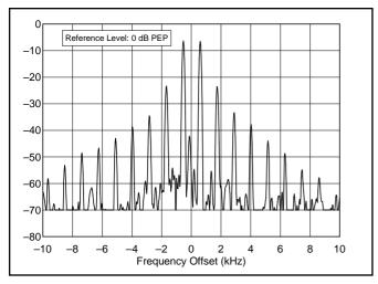
Figure 1—Worst-case spectral display of the unmodified IC-756 transmitter during two-tone intermodulation distortion (IMD) testing at 28.350 MHz. The worst-case third-order product is about 24 dB below PEP output, and the worst-case fifth-order product is about 34 dB down. The transceiver was being operated at 100 W output. (See text for additional details.)
