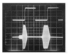
Figure 3—CW keying waveform for the unmodified IC-756 showing the first two dits in full-break-in (QSK) mode. The equivalent keying speed is 60 WPM. The upper trace is the actual key closure; the lower trace is the RF envelope. Horizontal divisions are 10 ms. The transceiver was being operated at 100 W output at 14.2 MHz. Note that the first dit is somewhat shortened. This is much less evident in semi-break-in mode.
