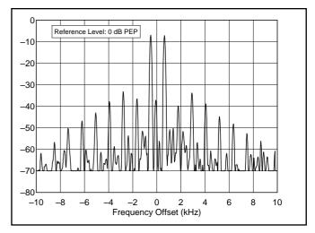
Figure 2—Spectral display of the unmodified IC-756 transmitter during two-tone intermodulation distortion (IMD) testing at 50.2 MHz. The worst-case third-order product is approximately 37 dB below PEP output, and the worst-case fifth-order product is approximately 33 dB down. The transceiver was being operated at 100 W output. (See text for additional details.)
