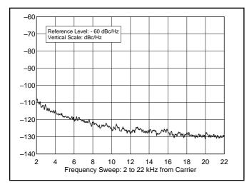
Figure 4—Worst-case tested HF spectral display of the unmodified IC-756 transmitter output composite-noise testing at 3.5 MHz. Power output is 100 W. The carrier, off the left edge of the plot, is not shown. This plot shows composite transmitted noise 2 to 22 kHz from the carrier.
