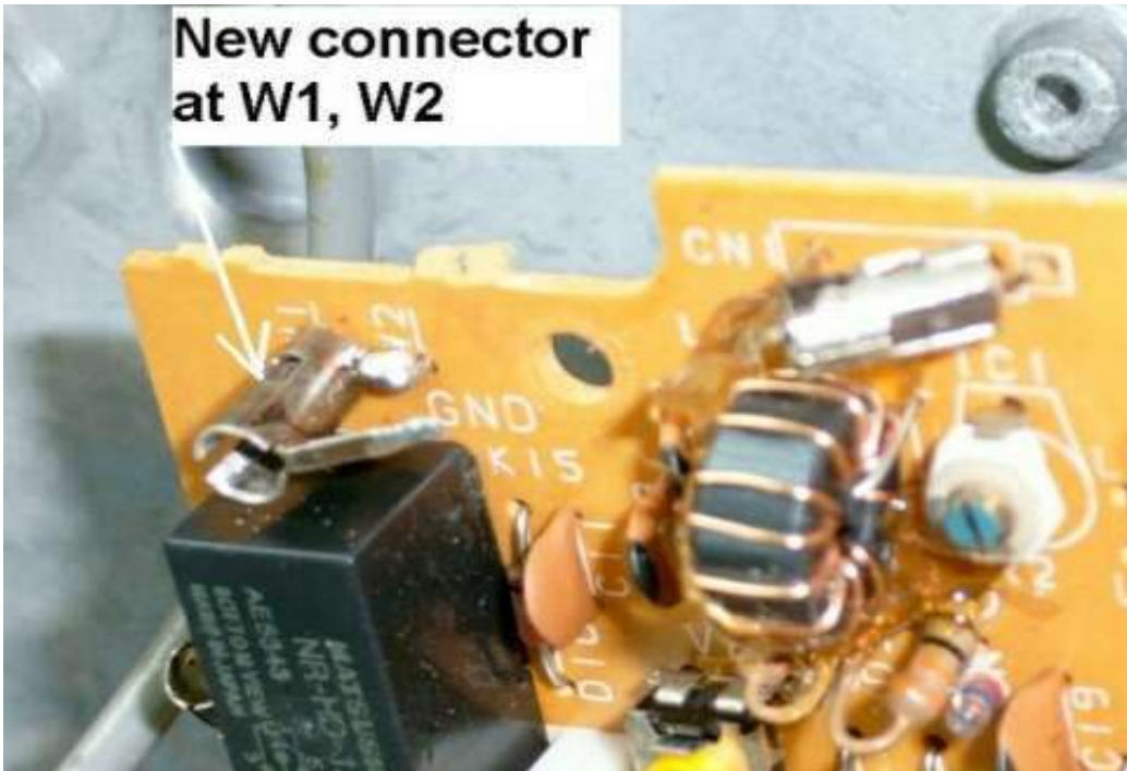
The first coaxial connector was installed. It's center contact is soldered at W1, outer (shield) at W2 (gnd). Note its positioning. The outer contact connection will be soldered later at a grounding tab/eyelet fixed by the (later installed at the hole) screw.
