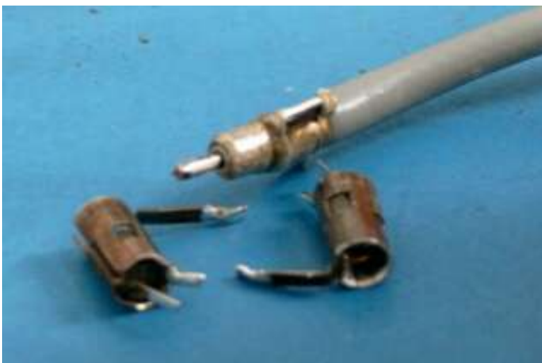
The two female coaxial connectors and the short length of coaxial cable (with male connectors) which need to be added. A grounding eyelet will also be needed.
