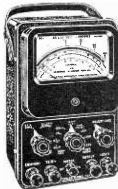
UNIVERSAL TAYLORMETER, Model 50A. 40 ranges. Sensitivity 1,000 ohms per volt, D.C. and A.C. First grade accuracy. Price £15.15.0.
