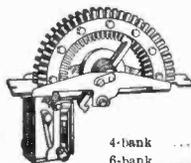
4- or 6-bank, 26 constants. Have various applications including a automatic tuning. circuit selection, etc. Operates on 25-50v.
