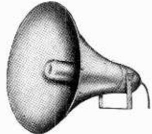
The new 42REH has advantages of complete weather-proofness, smaller overall length, better weight distribution and consequently greater ease in handling, which make this one of the most popular of the new F.I. loud-speakers. The horn is designed for use with the standard F.I. L.S.7 Unit and allows for this unit to be driven to 12 watts input. A spun aluminium cover over the unit has room for housing a suitable matching transformer.
