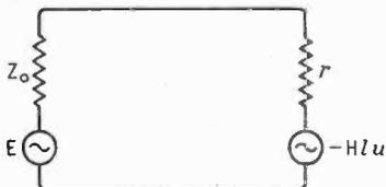
Let the coil resistance be  $r$  and the source have internal impedance  $Z_0$ , then applying Kirchhoff's law to the driving circuit, and substituting for  $I$  from (2),
