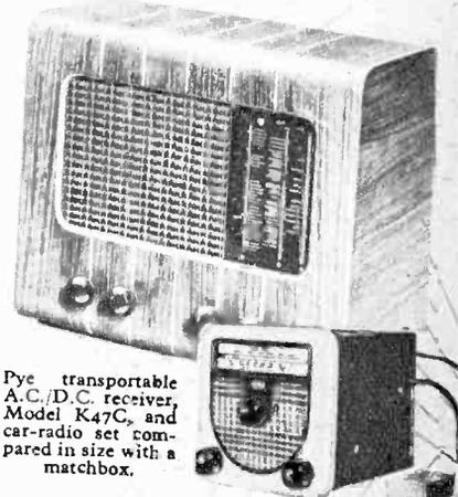
Pye transportable A.C./D.C. receiver, Model K47C, and car-radio set compared in size with a matchbox.
