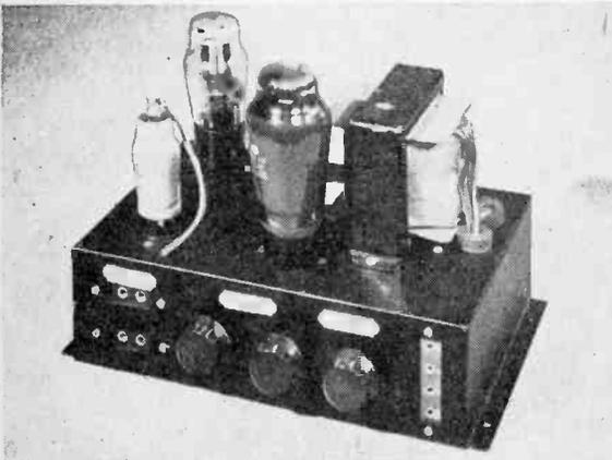
**10-watt AUDIO AMPLIFIER.** Dimensions 9½" x 6½". Overall height 6½". Two Channel Input. Tone Control. Heavy duty Output Transformer matched to 3, 8 and 15 ohms. Valves EF36, 5Z4, KT66. Intended for the record enthusiast. Highest possible efficiency, overall gain, stability and equality of reproduction. Eminently suitable for Concert Work, booster amplifier, standby for amateur transmitters, paging system, etc. **£8.8.0**
