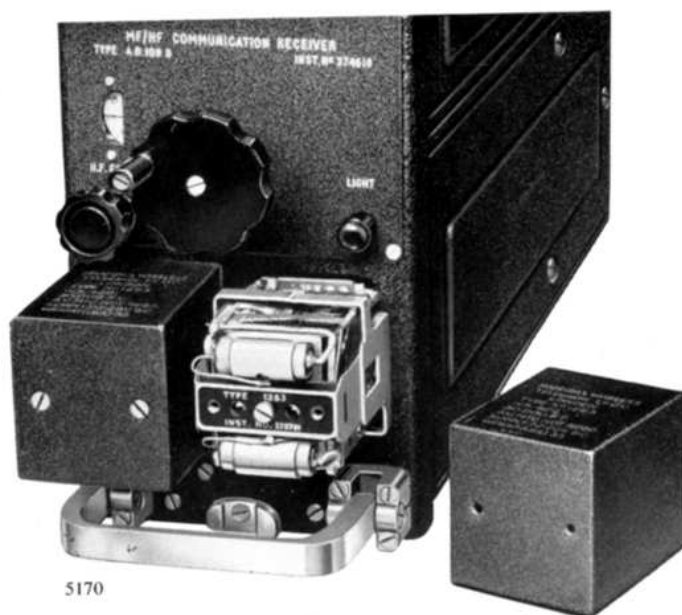
The receiver, ready for remote control operation, fitted with Type 1263 Controller Switch Drive Motors.
