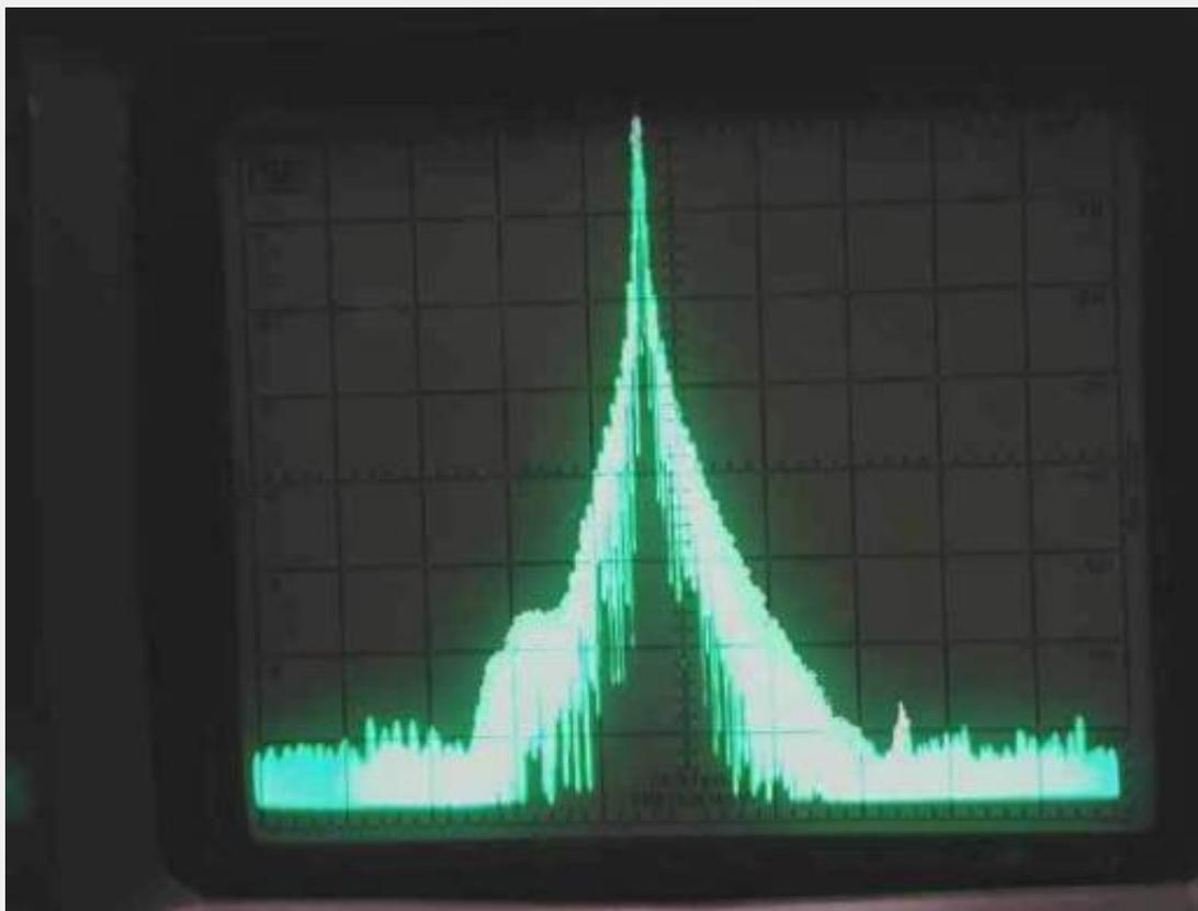
The FT1000-MP is approximately -50dB at 1kHz. It is 8 dB worse than the already "hard" 751A, and has a "click plateau" below the carrier frequency that hovers around -55dB for around 500Hz bandwidth.
