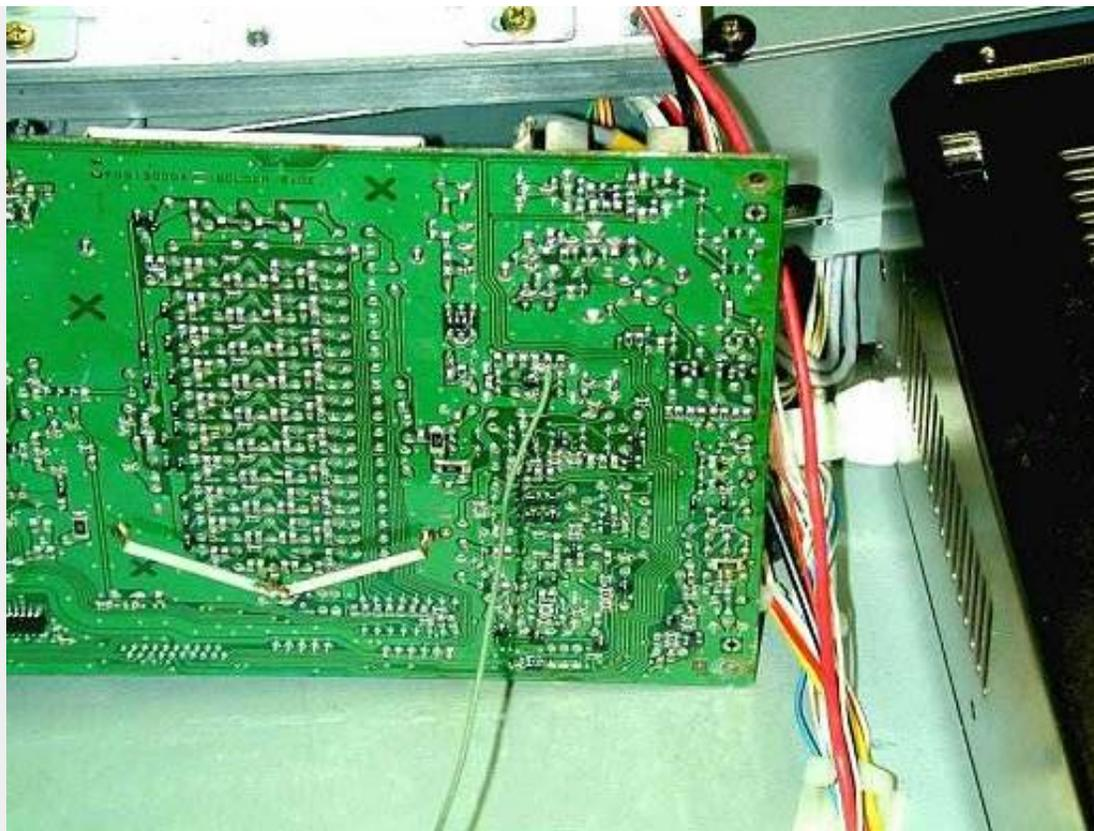
6. I added the green wire you see above. I tacked it on a foil pad by laying the wire across the point where two chip components soldered in, as shown below:
