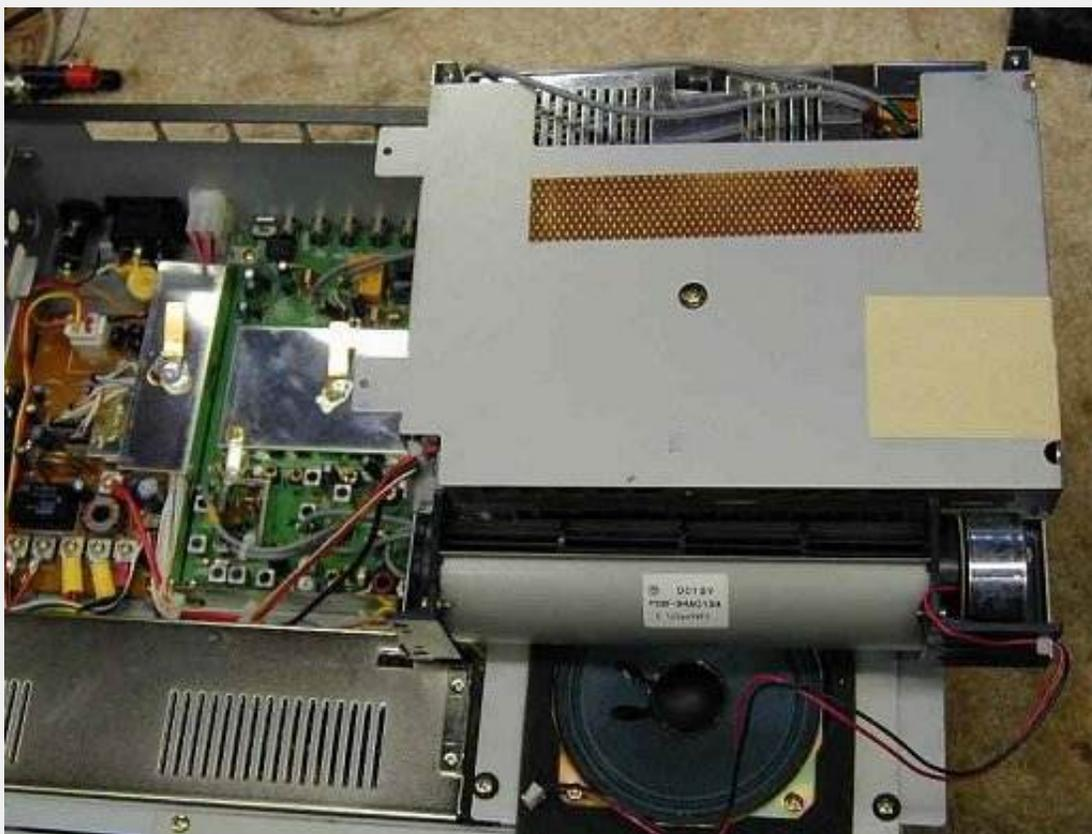
4. The RF board is the green-colored board you see above. There are several screws holding that board down, and two screws on a rear panel DIN connector that is mounted on that board. The board will freely move when you remove ALL the screws. Do NOT pry or force the board out, if you have to pry you missed a screw!
