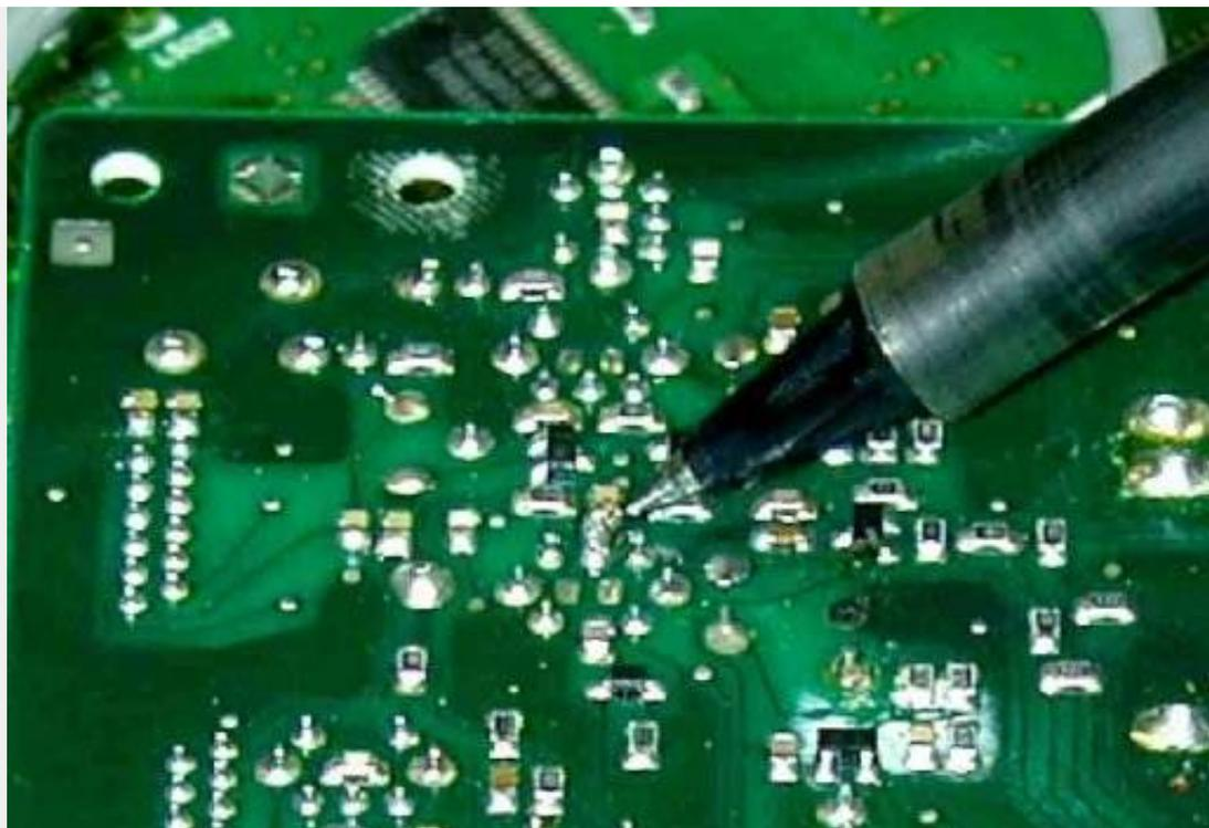
Note the FET above and to the left of the pen, and the IF transformer (two transformer shield connections and five electrical pin-outs, with an unused pad-set for a surface mount device in the center of the transformer leads) below the pen. The connection point for a new small insulated wire is the chip capacitor (C2148) pad that also connects to the center pin of the top three in-line pins of the IF transformer.
