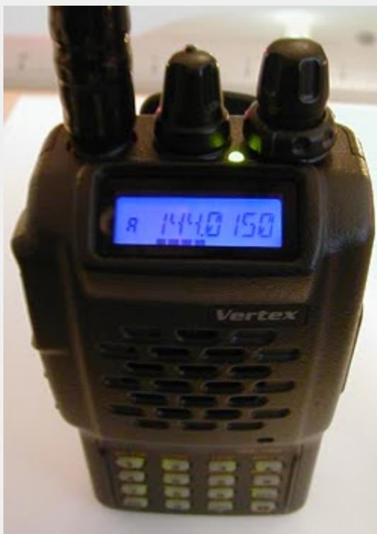
My VX-150 with the LCD display LED changed to Blue. The original LED was removed and replaced with a blue SMT LED (1206 size). R1239 (220Ohm) was removed and replaced with a 0 Ohm resistor.
