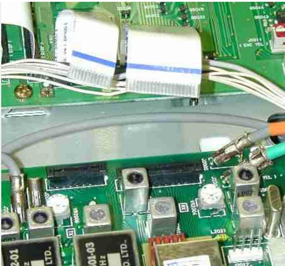
10. Remove the mounting screws and flip the IF board exposing the bottom:
