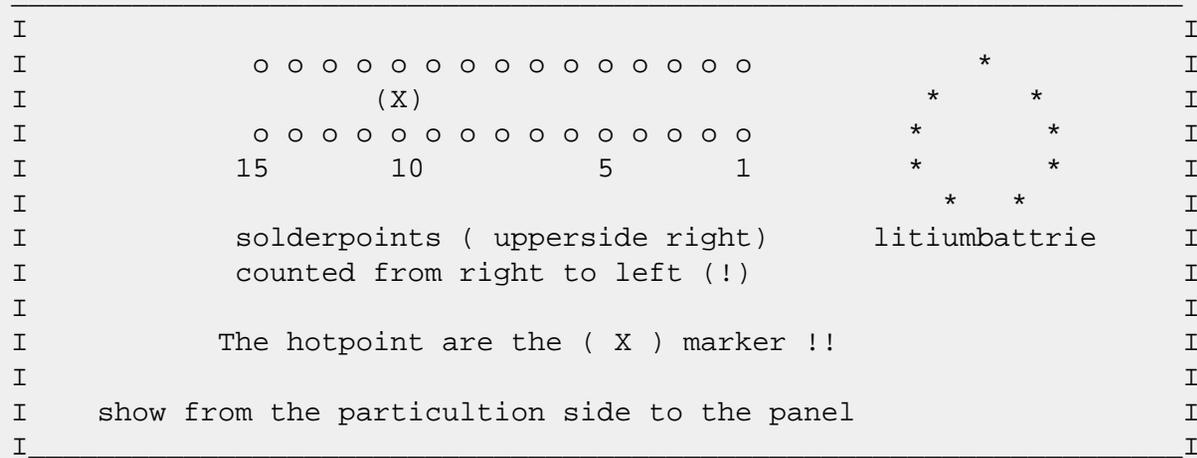
9. If you want only to open the RX , you must be have follow solder- points at this place are close in the area : 10 , 9 , 6, 4, 3, 1 That the version in DL if you can open the RX only by software Reset and the keysteps : press REV+VFO/MR and switch on the TRX in the same time.
