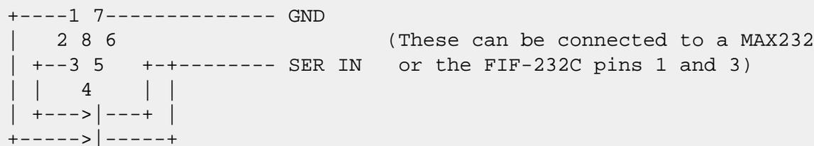
You can wire 1 and 3 together first, then through 1 diode, but that disables the UP and DOWN buttons.
