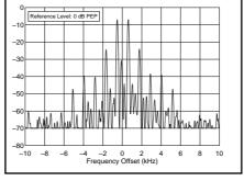
Figure 2—Worst-case VHF/UHF spectral display of the FT-100 transmitter during two-tone intermodulation distortion (IMD) testing. The worst-case third-order product is approximately 25 dB below PEP output, and the worst-case fifth-order product is down approximately 40 dB. The transceiver was being operated at 100 W PEP output at 50.2 MHz.
