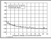
Figure 4—Worst-case HF spectral display of the FT-100 transmitter output during composite-noise testing. Power output is 100 W at 3.520 MHz. The carrier, off the left edge of the plot, is not shown. This plot shows composite transmitted noise 2 to 22 kHz from the carrier.
