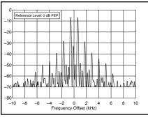
Figure 1—Worst-case HF spectral display of the FT-100 transmitter during two-tone intermodulation distortion (IMD) testing. The worst-case third-order product is approximately 30 dB below PEP output, and the worst-case fifth-order product is down approximately 40 dB. The transceiver was being operated at 100 W PEP output at 24.95 MHz.
