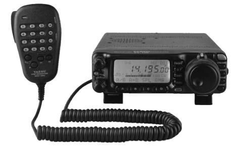
the desired button without also actuating an adjacent button. The important **UP** and **DWN** buttons—used to change bands—are sand-wiched between the **MODE** and **FUNC** buttons. The **MODE** button steps through the operating modes. The **FUNC** button accesses the menus. More on those later.
