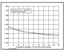
Figure 5—Worst-case VHF/UHF spectral display of the FT-100 transmitter output during composite-noise testing. Power output is 20 W at 432.02 MHz. The carrier, off the left edge of the plot, is not shown. This plot shows composite transmitted noise 2 to 22 kHz from the carrier.
