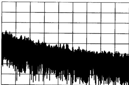
Figure 3—Spectral display of the Yaesu FT-840 transmitter output during composite-noise testing. Power output is 100 W at 3.5 MHz. Vertical divisions are 10 dB; horizontal divisions are 2 kHz. The log reference level (the top horizontal line on the scale) represents  $-60$  dBc/Hz and the baseline is  $-140$  dBc/Hz. The carrier, off the left edge of the photograph, is not shown. This plot shows composite transmitted noise 2 to 20 kHz from the carrier.
