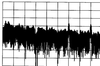
Figure 5—Spectral display of the S & S Engineering ARK 40 transmitter output during composite-noise testing. Power output is 3.6 W at 7 MHz. Vertical divisions are 10 dB; horizontal divisions are 2 kHz. The log reference level (the top horizontal line on the scale) represents 60 dBc/Hz and the baseline is 140 dBc/Hz. The carrier, off the left edge of the photograph, is not shown. This plot shows composite transmitted noise 2 to 20 kHz from the carrier.
