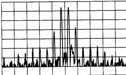
Figure 1—Worst-case spectral display of the Yaesu FT-840 transmitter during two-tone intermodulation distortion (IMD) testing. Worst-case third-order product is approximately 28 dB below PEP output, and the fifth-order product is approximately 49 dB down. Vertical divisions are 10 dB; horizontal divisions are 2 kHz. The transceiver was being operated at 100 W PEP output at 14 MHz.
