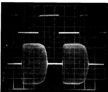
Figure 4—CW-keying waveform for the S & S Engineering ARK 40. The upper trace is the actual key closure; the lower trace is the RF envelope. Horizontal divisions are 10 ms. The transceiver was being operated at 5 W output at 7 MHz.
