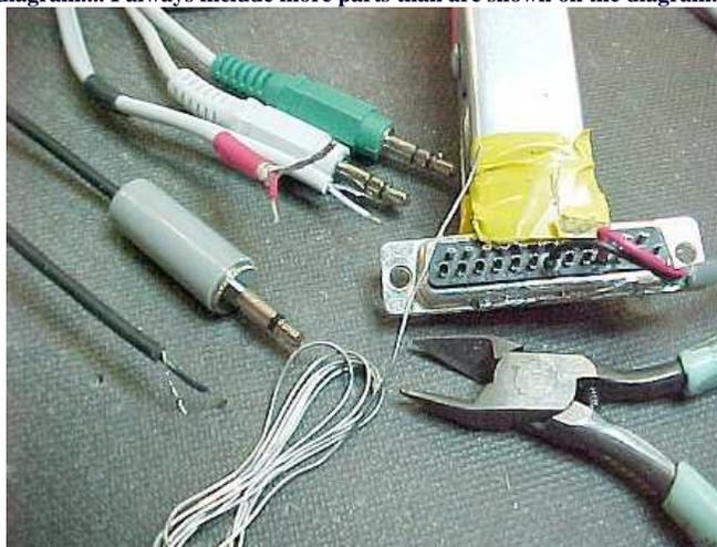
Carefully follow the diagram and begin the assembly of our interface by dressing the cable ends first.
