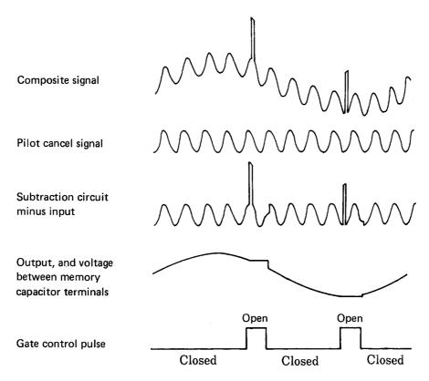
Note: The pilot cancel signal is given as sinusoidal in this explanation, but in the actual application circuit, pilot cancel is performed by a triangular wave.
